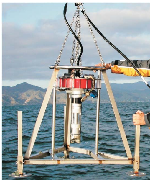
Figure 1: The SPI-Scan instrument used to obtain high-resolution in situ sediment profile images
