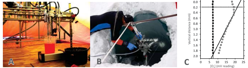
Figure 3. Two photographs showing (A) a Unisense lander setup with 4 microelectrodes and (B) a dive hole in the ice cover of Lake Fryxell through which the tethered lander was lowered to the lake floor. A diver moved the lander away from the ice hole to a 9 m-deep site. After deployment, the lander measured time series of O 2 concentration microprofiles across the upper 2-mm layer of benthic cyanobacterial mats. (C) Two example O 2 concentration (electrode mV reading) microprofiles measured 10 Dec, 1345 h (open squares), and 11 Dec 2006, 0303 h. The solid line indicates a linear fit through the sub-peak profile. The slope of this fit was used as proxy for the downward O 2 flux (see Figure 4 ). The dashed line indicates the mat surface.
