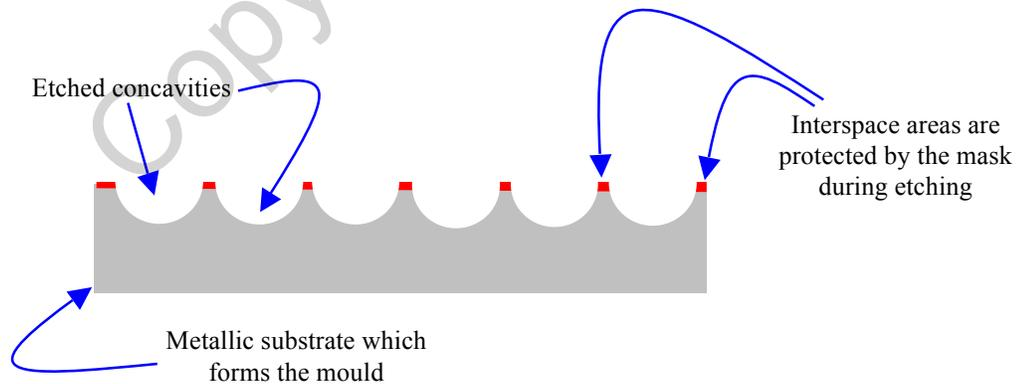
**Figure 29:** In his 1926 patent, Ernst describes the use of an acid resistant mask to support the formation of a metallic mould. Once the mask has been deposited, a suitable acid is used to etch the concavities. Subsequently, a set of lenticules may be created by, for example, pressing an appropriate malleable transparent material into the mould.
