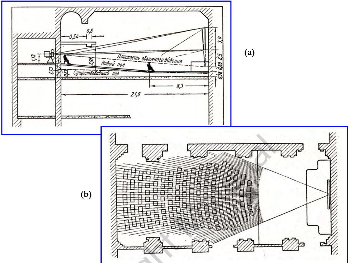
**Figure 26:** Russian cinema layout diagrams in side elevation (a) and plan (b) views. Also look ahead to Figure 42. (Diagrams reproduced from Ivanaov [1956].)
