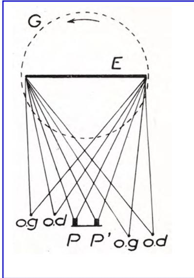
**Figure 38:** Diagram (a) provides a further insight into the operation of the Cyclostereoscope. Here,  $P$ - $P'$  denotes the locations from which the left and right stereo views are projected. Locations  $og$  and  $od$  indicate exemplar positions from which the 3D image may be observed. See text for discussion. In (b) a view of an image as seen through the barrier.
