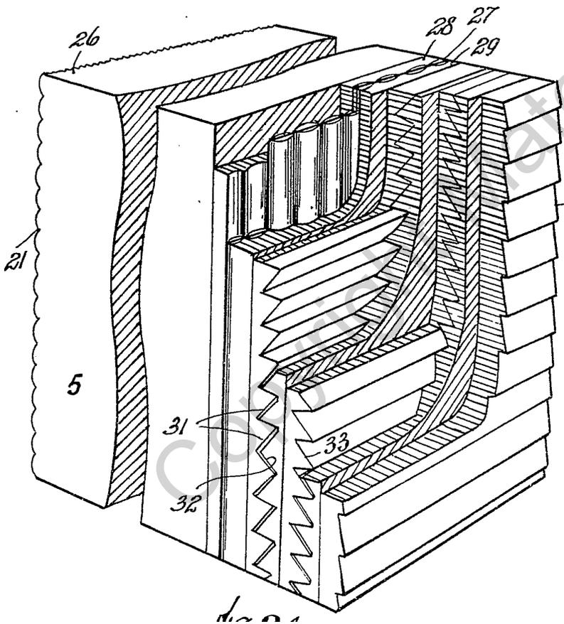
**Figure 41:** A cut away fragment of the optical structure designed by Gabor to provide glasses-free 3D cinema to audiences located on two tiers ('pit' and 'circle'). Notice that three mirror arrays are now employed (elements 31, 32 and 33). Unfortunately in the 1940's the implementation of such a structure with useful dimensions would have been extremely challenging. See Chapter 5 for discussion. (Reproduced from British patent 541,751.)
