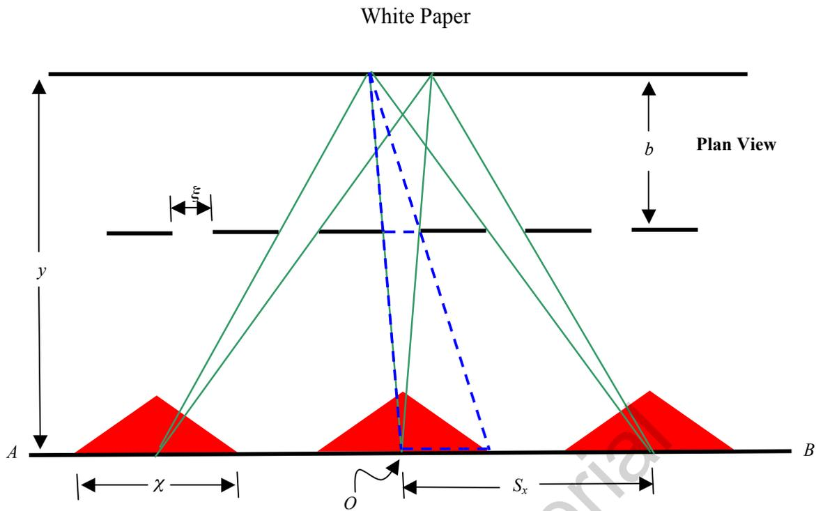
**Figure 14:** Illustrating the basic geometry giving rise to regions of visibility (depicted in red) for a point source located at  $O$ . In practical situations these visibility profiles have a more complex shape.
