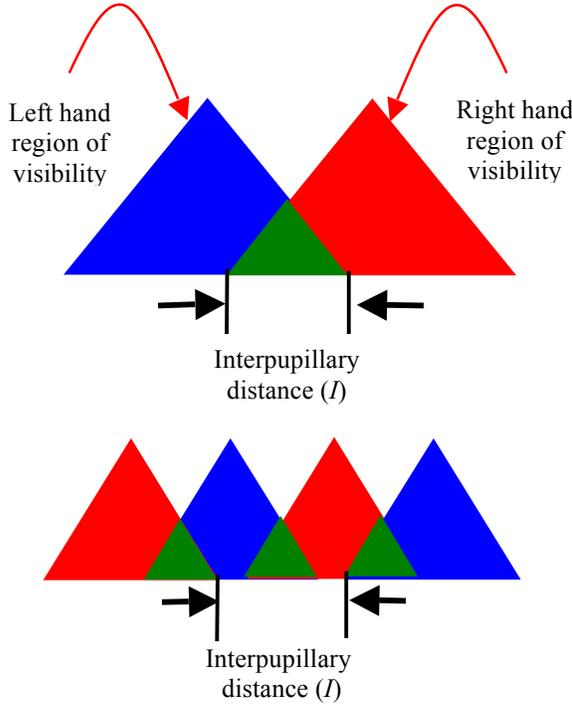
**Figure 18:** Simplified diagrams indicating the relationship between indicative viewing zones and interpupillary distance for furthest viewing distance (top) and smallest viewing distance (bottom). The green triangles indicate regions in which the left and right stereo views are simultaneously visible.
