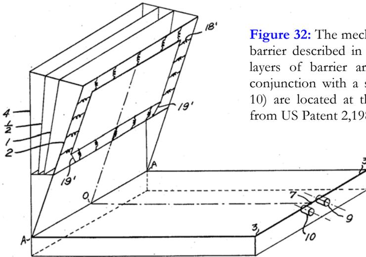
**Figure 32:** The mechanically complex multi-layer radial raster barrier described in Edmond Noaillon's 1937 patent. Three layers of barrier are employed (labelled 2, 1 and 1/2) in conjunction with a screen (4). The stereo projectors (9 and 10) are located at the rear of the auditorium. (Reproduced from US Patent 2,198,678.)
