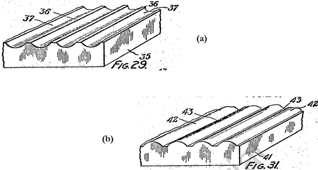
**Figure 28:** Greatly enlarged drawings of fragments of (a) plano-concave and (b) plano-convex lenticular panels. The fabrication of a range of micro-lens structures is described by Victor C. Ernst in a patent filed in 1926. (Reproduced from US Patent 1,849,036.)
