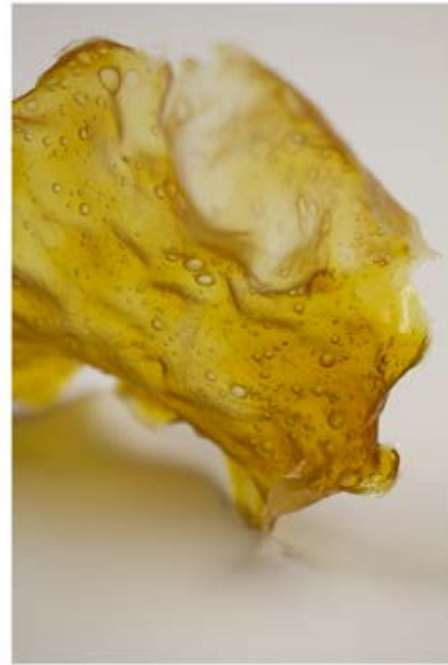
Experiment 14: THE YELLOW SEA starch, glycerol, turmeric powder and water texture: bubbled surface, brittle touch - no flexibility
