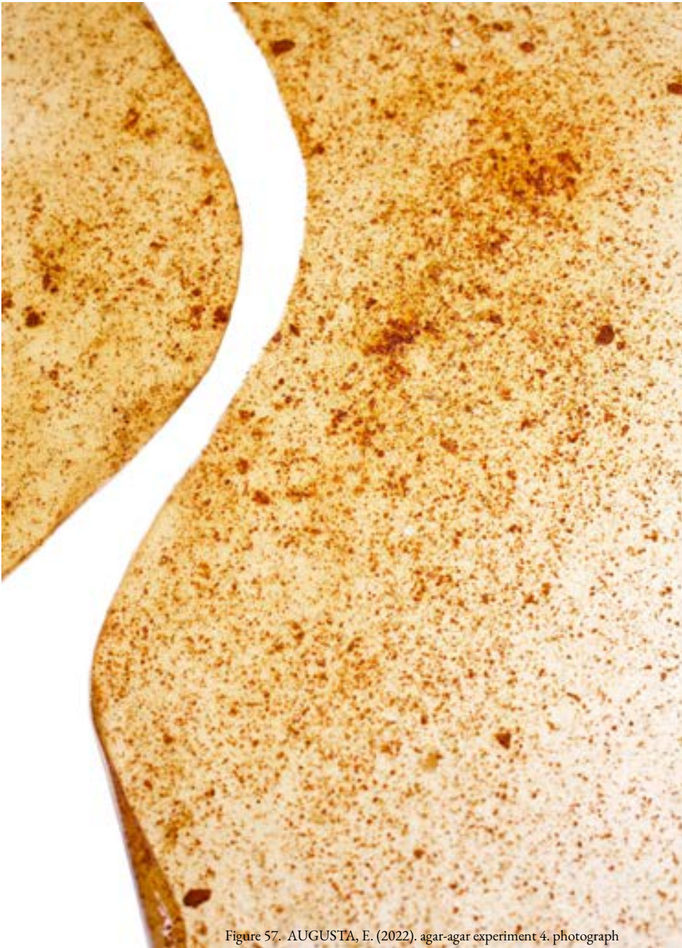
agar experiment four (left): agar, glycerol, water and mixed-spice blend texture: top side - coarse due to the spice powder, under side - rubbery with an adhesive quality
