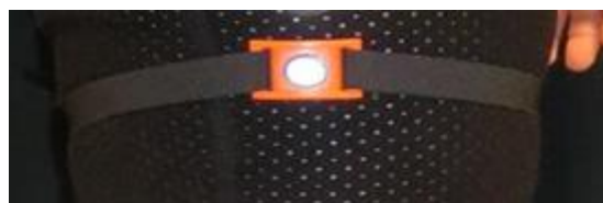
Figure 3. Inertial measurement unit with strapping
