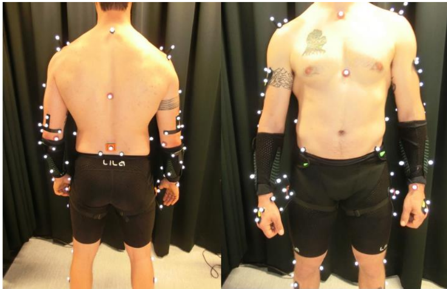
Figure 2. Attachment sites of retro-reflective markers for upper limb loading
