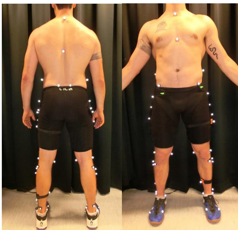
Figure 1. Attachment sites of retro-reflective markers and inertial measurement units with strapping for lower limb loading
