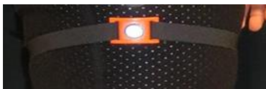
Figure 3. Inertial measurement unit with strapping
