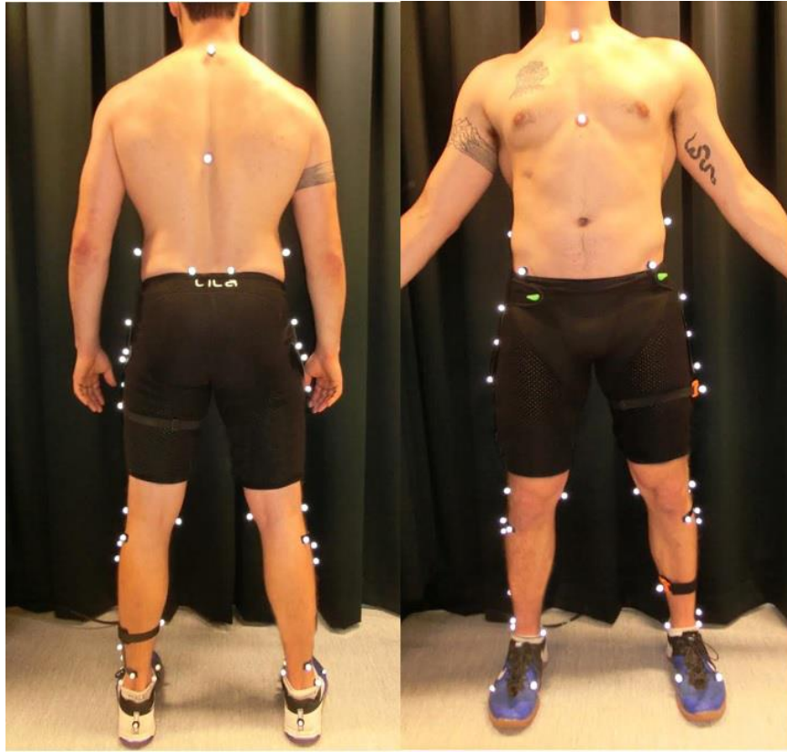
Figure 9. Marker set-up and inertial measurement unit attached to the mid-point of the thigh and shank of the left leg.
