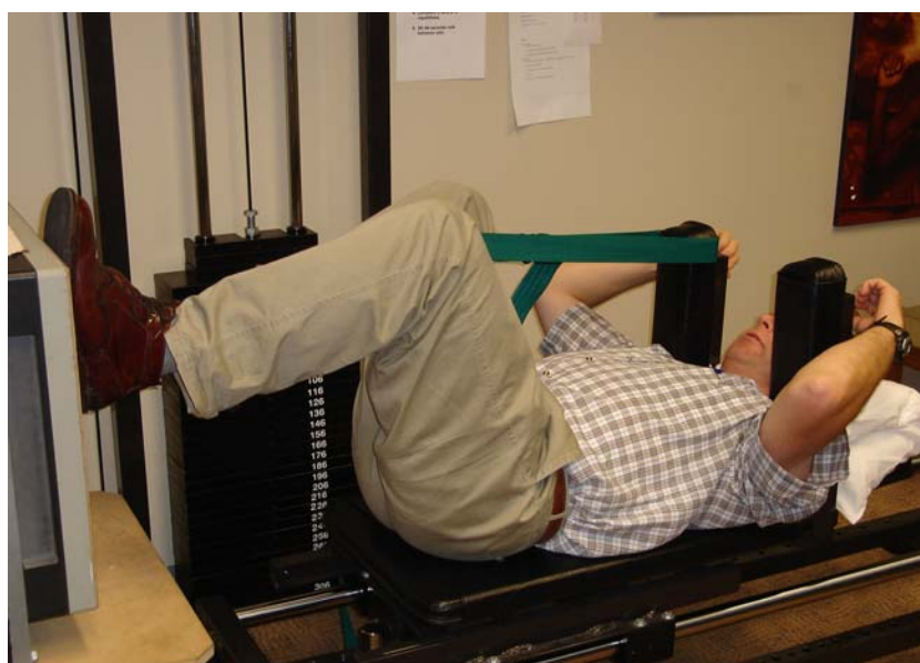
Figure 3.4 Starting position for testing the left leg of the participant on the modified supine leg press machine.
