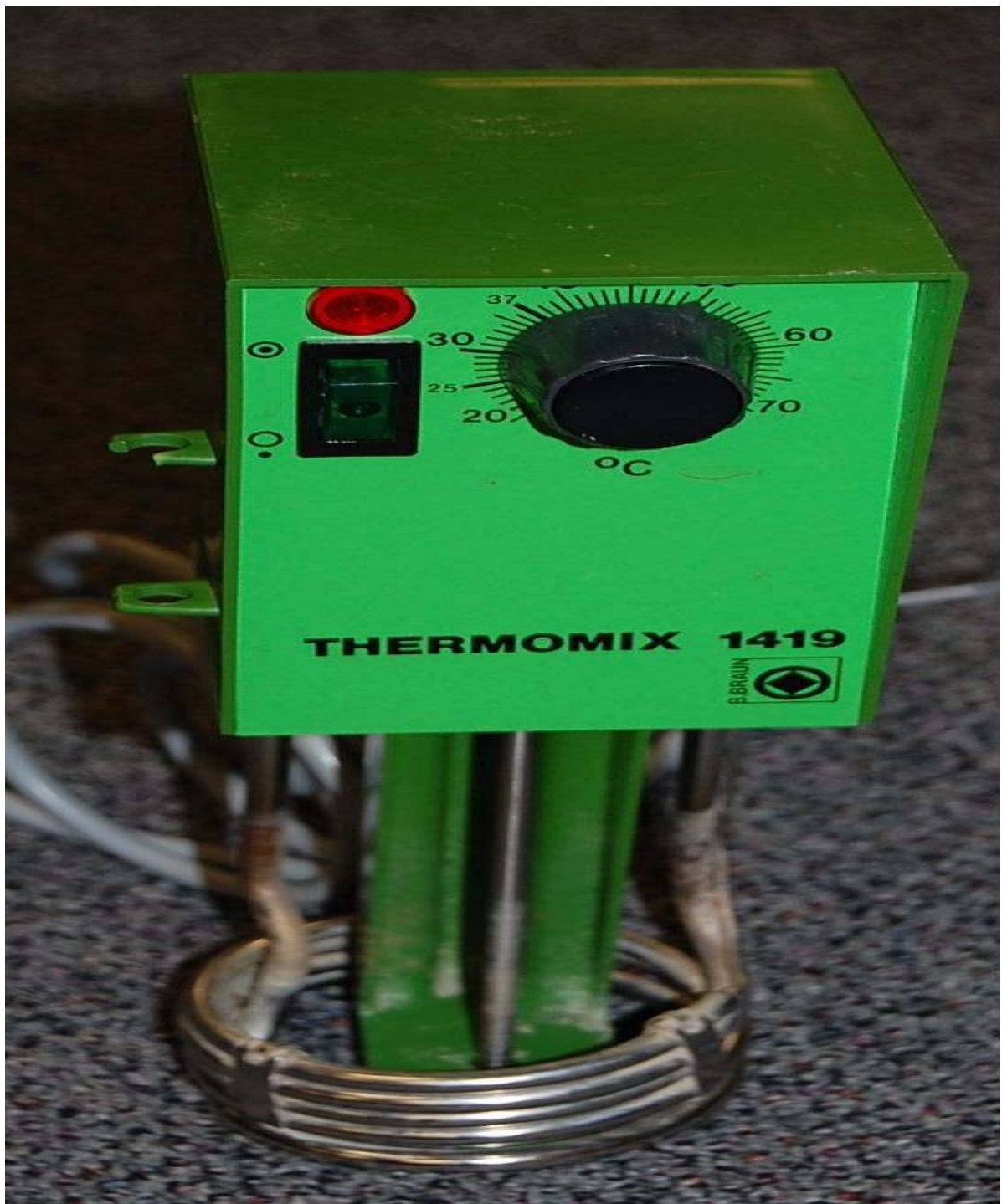
Figure 3.3 - B.Braun Thermomix 1419 used for Temperature control (Adapted from Manual of B.Braun Thermomix)
