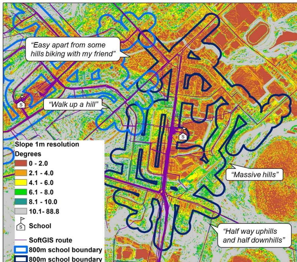
Figure 21. Inspection of slope data around one of the schools where the participants perceived slope as a barrier in the softGIS survey.
