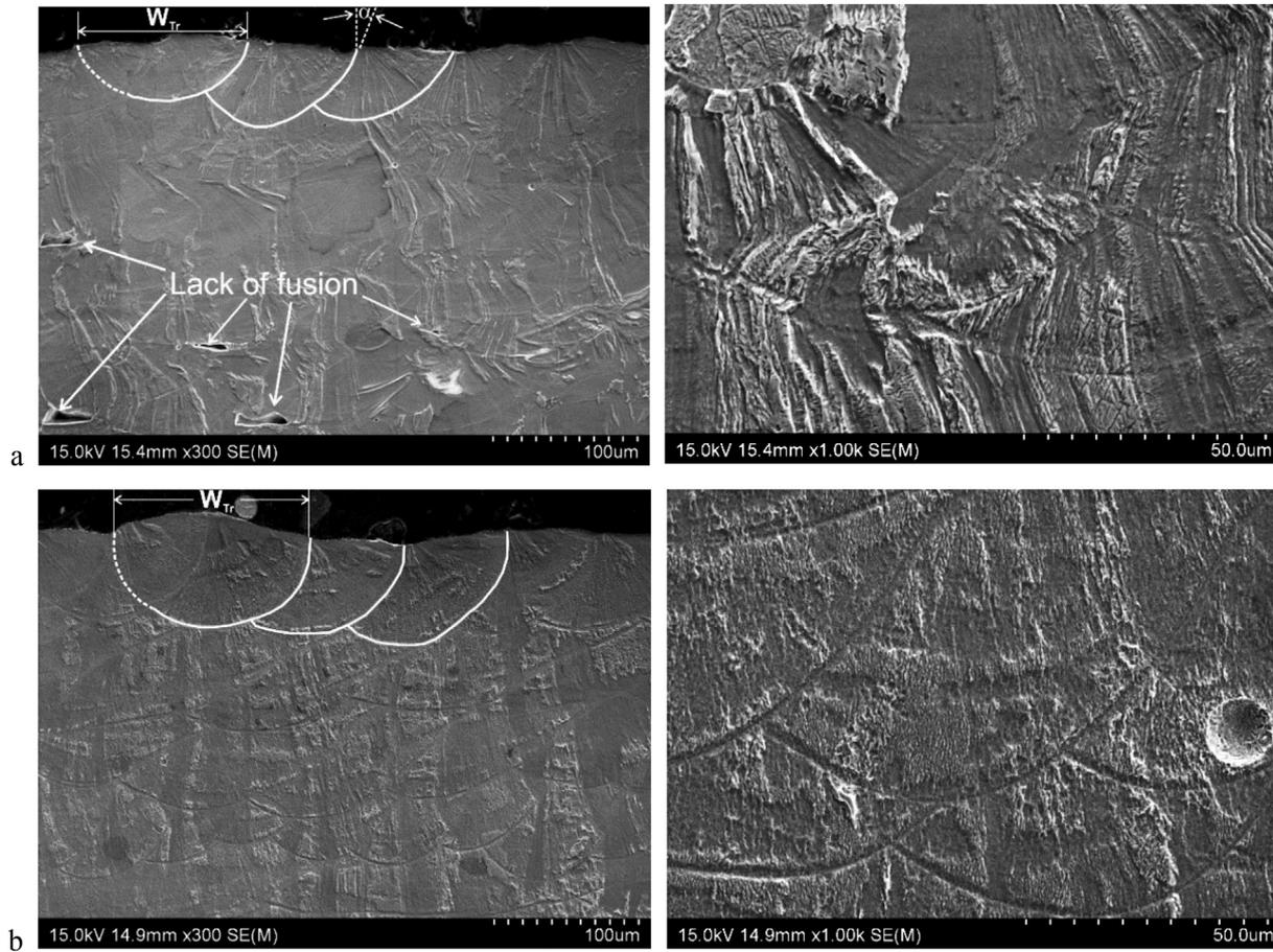
**Fig. 1.** SEM micrographs (left - low magnification, including the surface scan layer with three tracks outlined and right - higher magnification displaying track boundaries clearer): (a) 44 J/mm<sup>3</sup> and (b) 85 J/mm<sup>3</sup>. Note: a number of LOFs are pointed to in the left micrograph of (a) and a keyhole pore is present in the right micrograph of (b).
