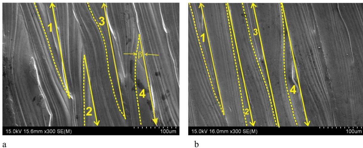
**Fig. 2.** SEM images of sample surfaces: (a) 44 J/mm<sup>3</sup> and (b) 85 J/mm<sup>3</sup> samples. Arrows point to scan direction along the track boundaries. For each arrow the shape of the area bounded by the arrow and dotted line indicates the partial melt pool at a time.
