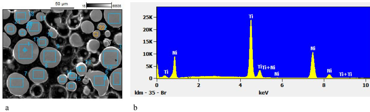
Fig. 3. EDS analysis of powder: (a) SEM image of powder showing area EDS in each powder and (b) a typical spectrum showing the Ti and Ni peaks.
