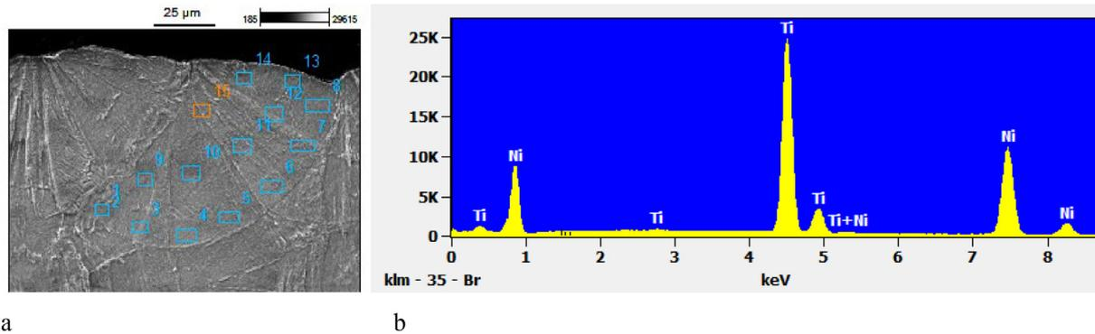
Fig. 4. EDS analysis of the 44 J/mm<sup>3</sup> sample: (a) SEM image illustrating the EDS areas in various locations in a track, 7 next to and along the track boundary (TB) and 7 inside the track, and (b) a typical spectrum showing the Ti and Ni peaks.
