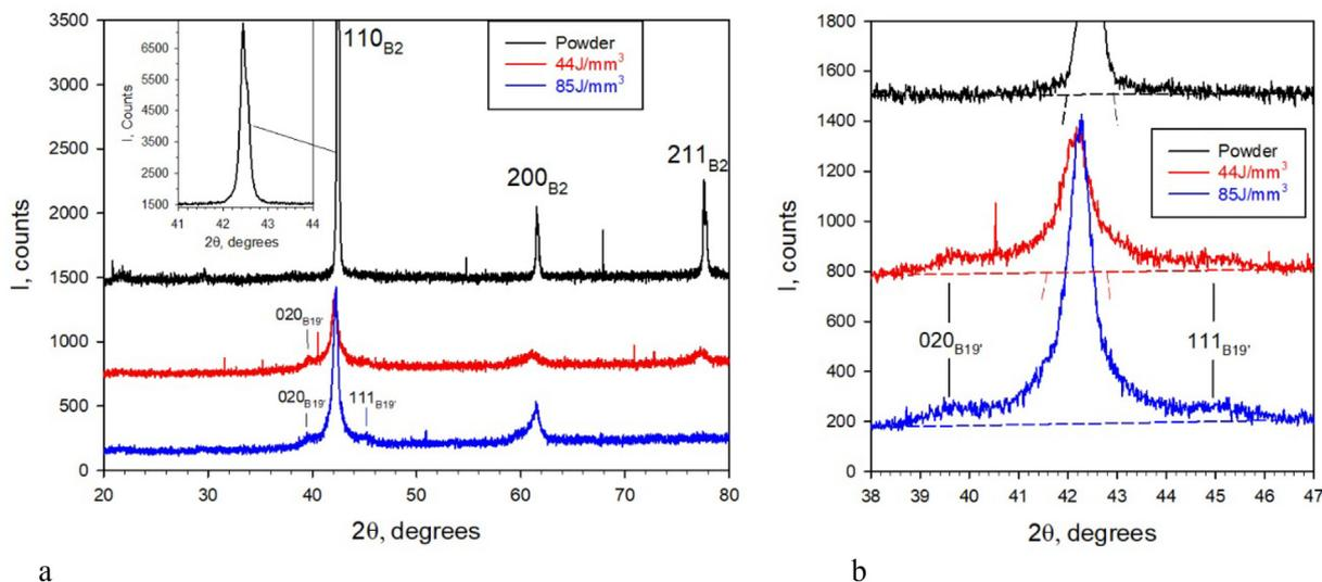
**Fig. 5.** X-ray diffraction patterns of powder,  $44 \text{ J/mm}^3$  and  $85 \text{ J/mm}^3$  samples: (a) pattern for  $2\theta$  from 20 to  $80^\circ$  with main diffraction peaks from B2 and weak diffraction peaks from B19' indicated, and (b)  $2\theta$  from 38 to  $47^\circ$  with background base lines indicated.
