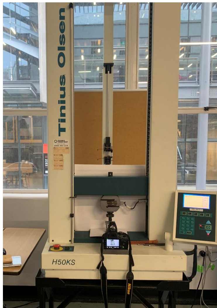
Fig. 3.12 Image capturing setup during compression testing (at AUT Mechanical Lab)
