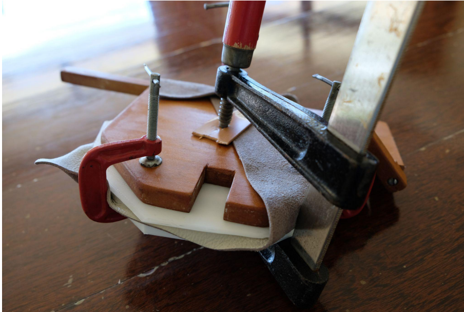
Fig 68. Wet forming the leather 'ripple'.
