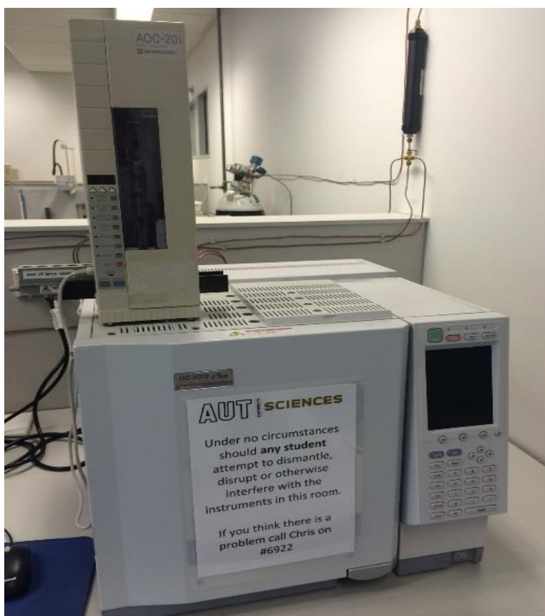
Figure 6 Shimadzu GC2010 gas chromatograph used in this study equipped with a Flame Ionisation Detector.
