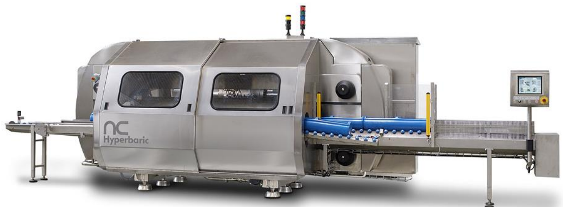
Figure 4 An example of a HPP instrument used (nc hyperbaric, hyperbaric 55).
