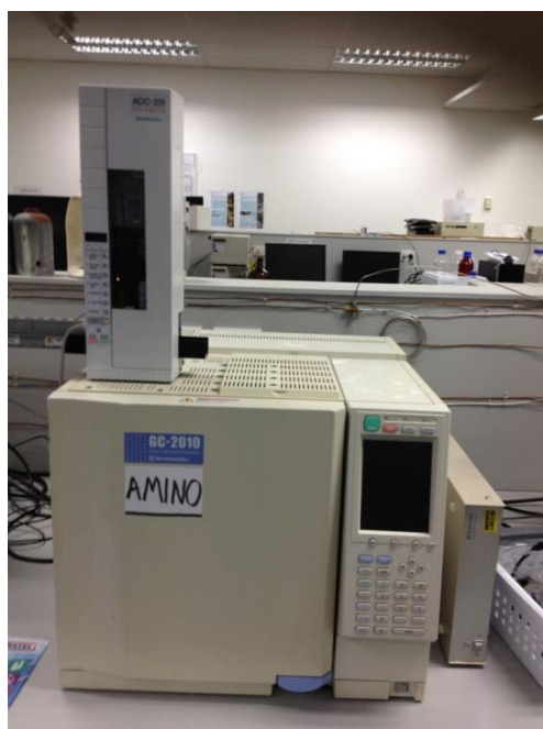
Figure 5 Shimadzu GC-2010 Gas Chromatograph with AOC-20i Auto Injector
