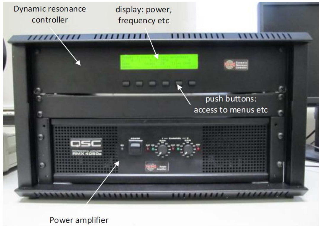
Fig.1-6. Power supply for the ultrasound transducer [1].
