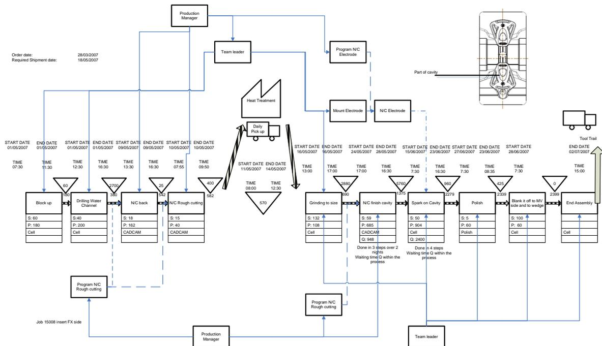
Figure 7: Current Value Stream Map of an insert
