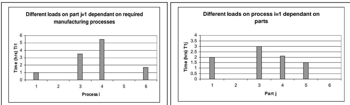
Figure 2: Process time of several processes for part  $j=1$ , Figure 3: Process time of several parts in the process  $i=1$  e.g. rough cutting
