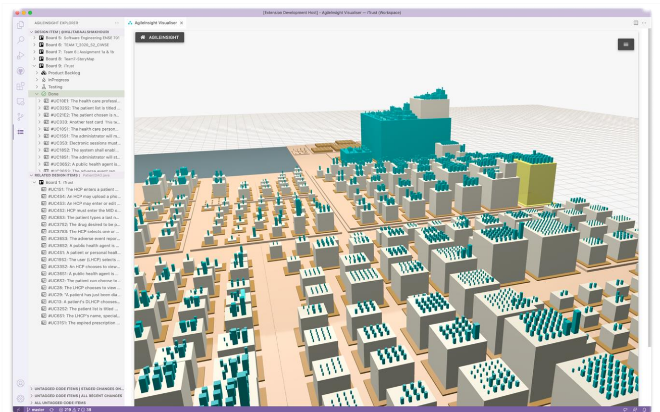
Figure 7.11: Bi-directional traceability in action showing design items revealed in side viewlet (lower left) after command invoked for a building of interest (yellow coloured).
