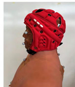
Figure 2 The headgear conditions tested during the tackles including no headgear, club-level headgear, and professional-level headgear. The headgear was purchased without the manufacturer's logo. Each headgear was International Rugby Board (IRB) approved.
