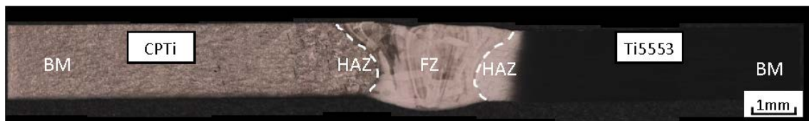
Figure 8.9. Microstructure of as-welded Ti5553-CPTi: LBW
