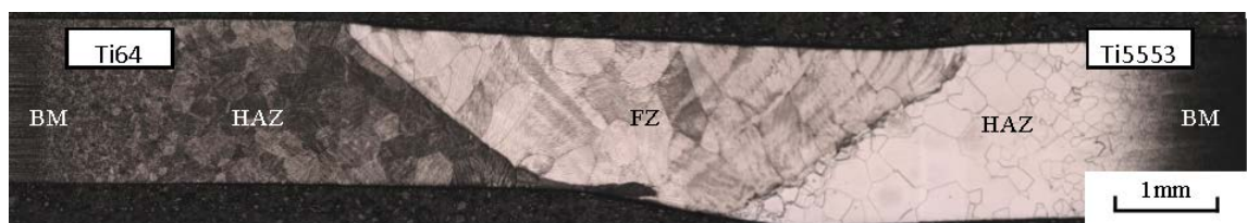
Figure 8.3. Microstructure of as-welded Ti5553-Ti64: GTAW
