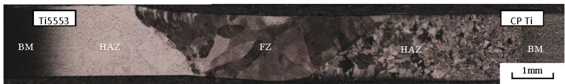
Figure 8.8. Microstructure of as-welded Ti5553-CPTi: GTAW
