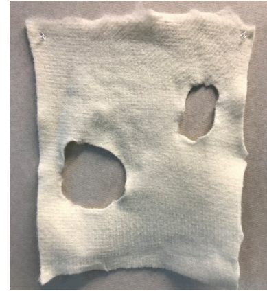
Machine Felted wool with controlled holes. The holes were made during the felting process to make them look finished and organic and that it looks like it was made into the textile rather than simply cutting out and leaving clean shape lines in the material. This first swatch is a thicker layer of felt using 1 whole Batt rather than the second that was trying to achieve a less rigid fabric that could drape and be worn. However that proved unsuccessful as the fabric can be pulled apart with slight pressure which would make it unsuitable for everyday wear. I do like how structured the 1st sample is and maybe this could be played with in laying through outfits?
