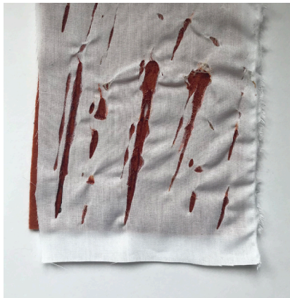
Soldering Iron Manipulated Synthetic Fabric. Using the Soldering Iron as an adhesive to join Fabrics.
