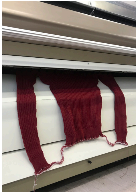
Figure 18: Jumper coming off knit machine
