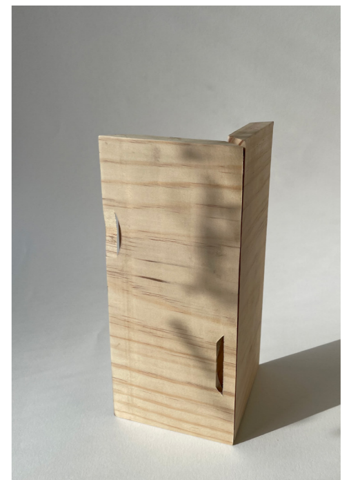
Figure 59. Saso, Denise. Investigating how the mitre panels join with a biscuit dowel and splined mitre. Auckland, New Zealand, 2024.
