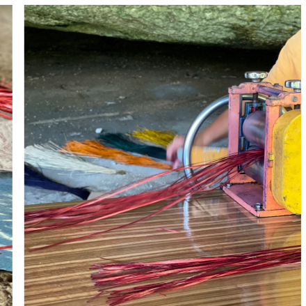
Fig. 12. Saso, D. Flattening the dyed tikog with a machine. 2023.
