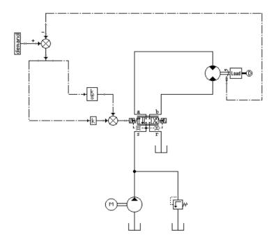
Figure 4.1 : Hydraulic test circuit
