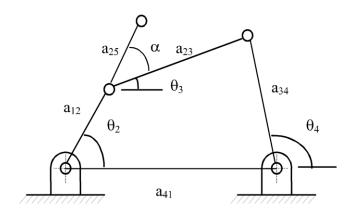
Figure 3.1 : Four bar mechanism
