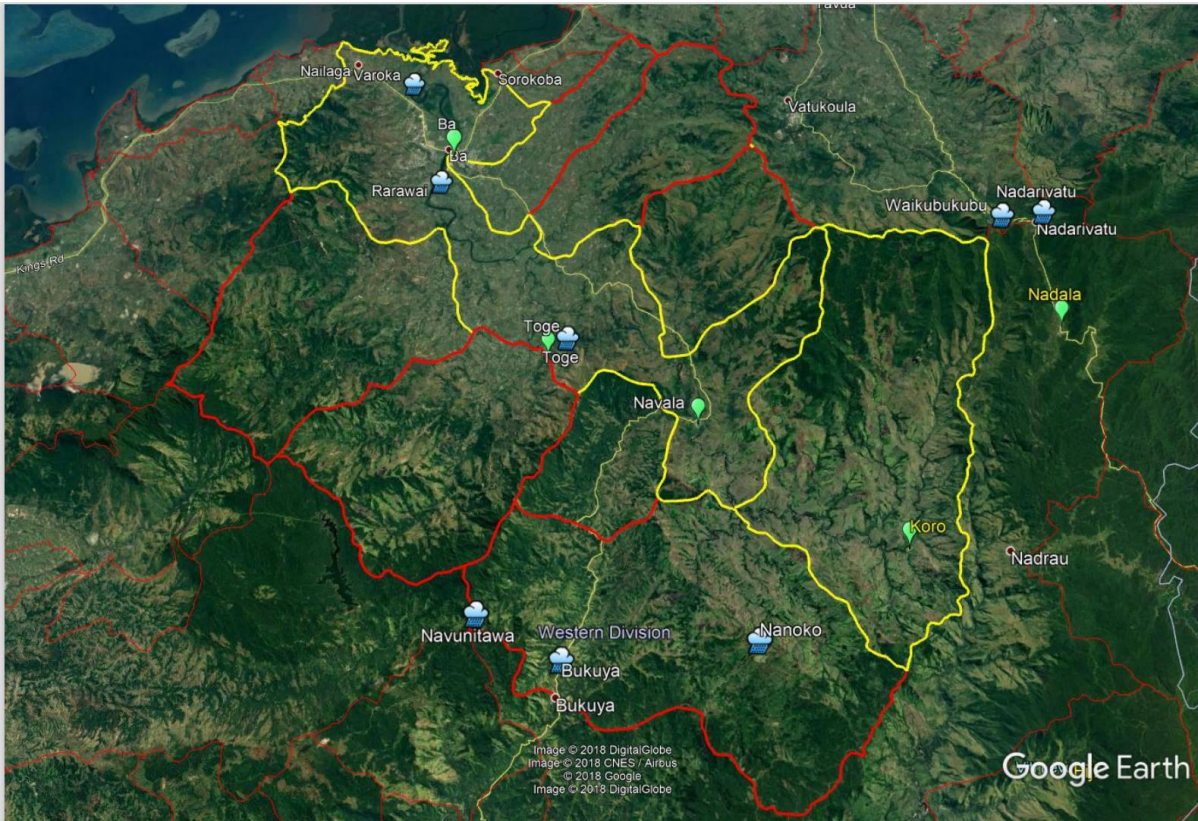
Figure 11 Location of telemetered stations and automatic weather stations in Ba Catchment. The stations are Varoka, Nailaga, Sorokoba, Rarawai, Navunitawa, Bukuya, Nanoko, Koro, Navala, Toge and Waikubukubu.
