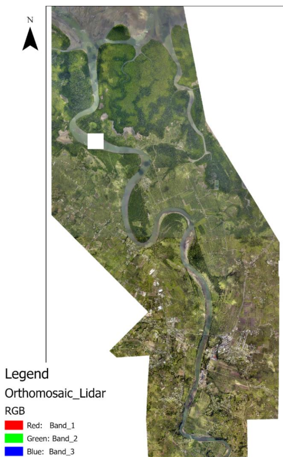
Figure 65 Orthomosaic of 434 LiDAR imageries to generate a DEM output
