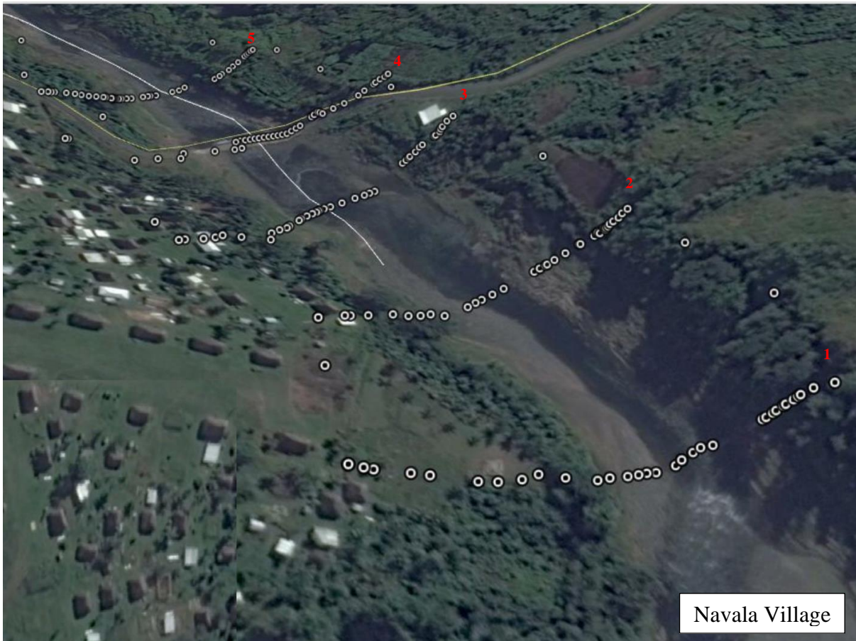
Figure 37 cross-section of estimated flood height at Navala Village. Cross section 4 is of the road and bridge into the village.
