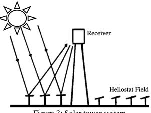
Figure 3: Solar tower system
