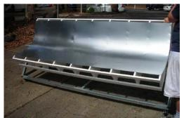
Figure 1: Small parabolic trough reflector (no absorber tube shown)
