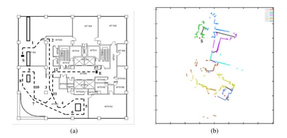
Figure 4.15: (a) The environment and path as used in Experiment 6 (Figure 3.12a). (b) Seven places (each with a different colour) were computed when Albot1 arrives at point 5 and after computing 37 local maps. Black lines denote exits crossed.
