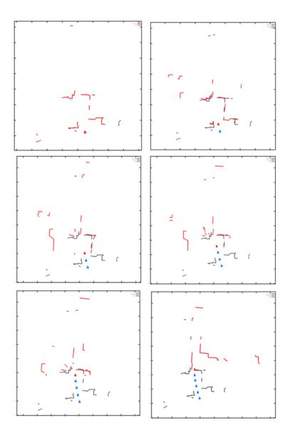
Figure 3.5: Albot1's first 6 local maps computed using the route shown in Figure 3.1: (top left) The first view accepted as the first local map. (the rest) Other local maps computed (in red) and each is superimposed onto the first local map (in black). The blue dots indicate Albot1's position where a view is accepted as a local map.
