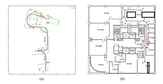
Figure 3.11: (a) The simplified trace map (intermediate points not shown). (b) Albot1 successfully returned home.
