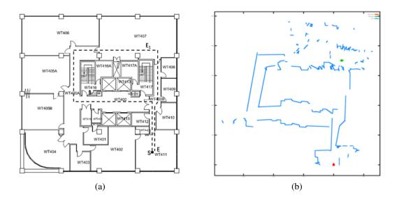
Figure 1.1: (a) A typical test environment. (b) Albot1's global map of the environment at E1.
