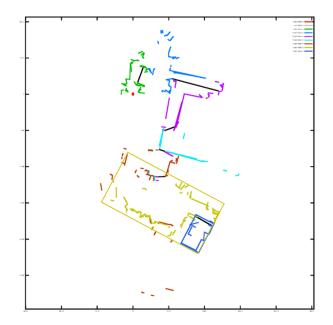
Figure 4.20: Computing the geometry of the last two places (in yellow and blue) allows Albot1 to detect that it is in the same place or not (see Figure 4.16).
