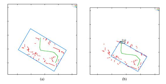
Figure 4.19: Computing the geometry of a place: (a) the outer boundary. (b) the inner boundary. The black rectangle indicates from where Albot1 enters into this place and the green line indicates the path Albot1 took inside this place.
