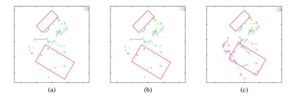
Figure 4.23: Albot1 continues exploring its environment and created three places, denoted in different colours: (a) green, (b) blue, and (c) purple.
