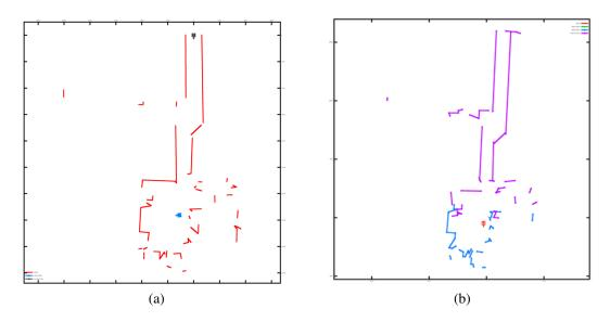
Figure 4.6: (a) The egocentric map computed prior to turning around at the bottom. (b) The enduring map computed by adding the new part of the egocentric map to its existing enduring map, and red point indicates where it exited the enduring map.
