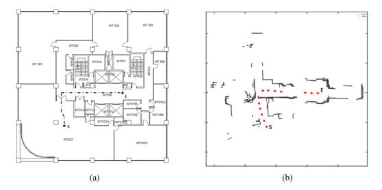
Figure 3.1: Experiment 1: (a) The environment and the route,  $S \rightarrow E$ . (b) Albot1's trace map (12 red dots) displayed with each local map superimposed.
