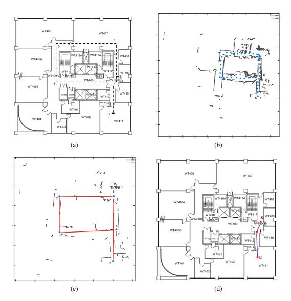
Figure 3.14: (a) The environment and the path (b) The trace map. (c) The simplified trace map with an intersection point detected. (d) Albot1 returned home using the short-cut.
