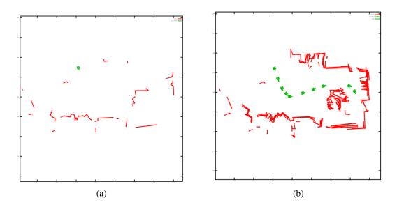
Figure 4.18: (a) Albot1 just entered into a new place, from Figure 4.17 (bottom row). (b) overlaying all local maps experienced in this place.
