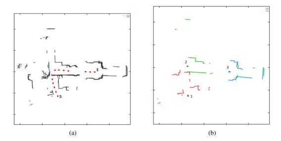
Figure 3.7: (a) Albot1's trace map. (b) Albot1's simplified trace map with each local map displayed in a unique color (intermediate points are not shown). Albot1 now re-tracing with 4 points rather than 12.
