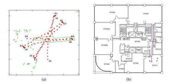
Figure 3.4: (a) The trace map (starting from S1-E1, S6-E6) displayed with its egocentric map, and (b) the result. Albot1's retrace path is  $S \rightarrow 1 \rightarrow 2 \rightarrow 3 \rightarrow 4$  it fails to reach 4.
