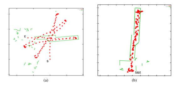
Figure 4.2: Experiment 2 repeated: (a) Albot1's egocentric map refreshed 6 times. (b) A single enduring map is computed. Red dots show Albot1's absolute position in the map.
