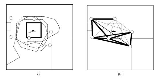
Figure 2.10: An example of a computed allocentric map using Brom et al.'s model. (a) shows the travelled trajectory (lines) in the test environment with 6 objects (empty circles). (b) shows the computed allocentric map with allocentric vectors (black solid lines). (Reproduced from Figures 16 and 20, Brom et al., 2012)
