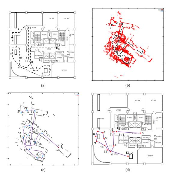
Figure 3.13: (a) The environment and the path. (b) The trace map superimposed with all the local maps (c) The simplified trace map (intermediate points not shown). (d) The result of Albot1 re-tracing home. It failed and stopped at point 12.
