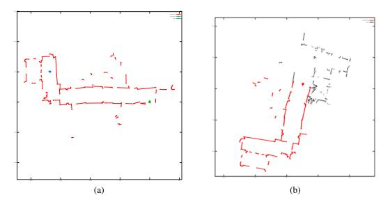
Figure 4.12: (a) The egocentric map computed prior to turning around at point 5. (b) The enduring map computed.
