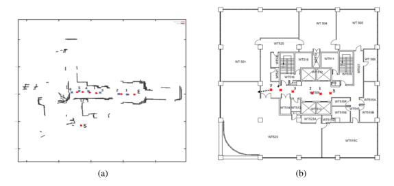
Figure 3.2: Result of Experiment 1: Albot1 failed to return home. The red dots show Albot1's re-tracing home.
