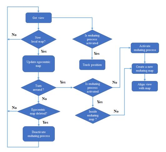
Figure 4.3: A flowchart of Albot1's cognitive mapping that computes both an egocentric map and an enduring map.
