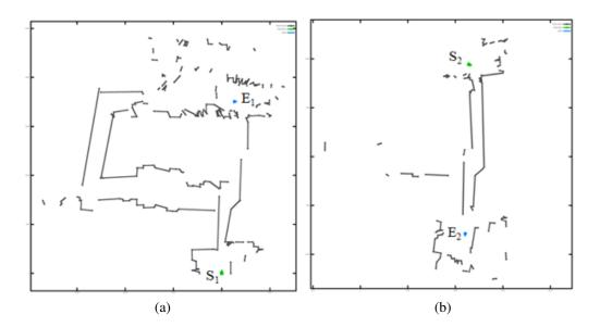
Figure 1.3: When Albot1 turns at E1, its existing egocentric map will start afresh building a new egocentric map. The previous one (left) could be kept to create a series of global maps computed.
