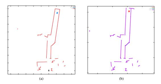
Figure 4.5: (a) The egocentric map computed prior to turning around at the top. (b) The enduring map computed and re-aligned with Albot1's current view looking down the corridor.
