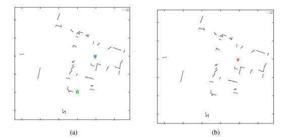
Figure 4.9: (a) The egocentric map computed prior to turning around at point 1. (b) The enduring map computed and re-aligned with Albot1's current view.
