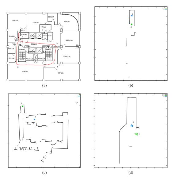
Figure 4.14: (a) The environment and the route traversed, (b) The enduring map computed after turning around at point 1, (c) The egocentric map computed at point 5, and (d) The egocentric map computed at point E.
