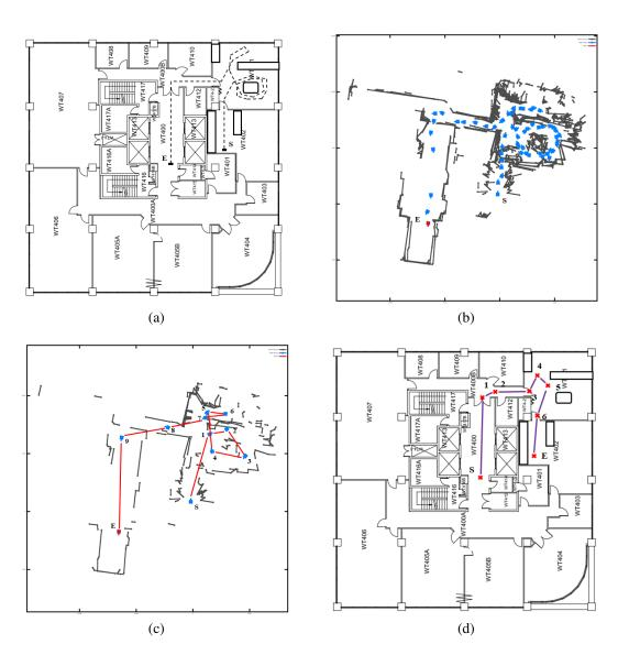
Figure 3.15: (a) The environment and the path taken. (b) The trace map. (c) The simplified trace map. (d) Albot1 returned home using a short-cut.
