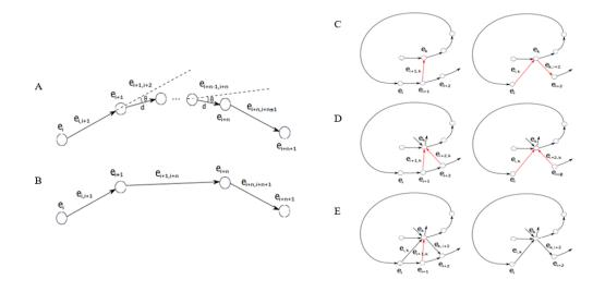
Figure 2.4: A and B show the adding of sparse sequential vertices and edges to both a. standard cognitive map and a compact cognitive map respectively. C - E show scene integration. When one revisits a familiar space, it removes the redundant vertices and edges. Red arrows indicate the loop closure edges. (Reproduced from Figures 2 and 4, Zeng & Si, 2019)
