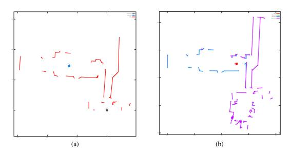
Figure 4.7: (a) The egocentric map computed prior to turning around on the left side of the corridor. (b) The enduring map computed again by adding the new part of the egocentric map to its existing enduring map.
