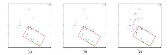
Figure 4.21: (a) Albot1 refreshes its egocentric map (in green) together with the geometry of the familiar place that it is in (the red rectangle). (b) Albot1 moves into a new place and identify that it is still part of the familiar place that it was in. (c) Albot1 moves into another new local place which is now no longer a part of its familiar place. A new exit, E', now appears on the geometry of the familiar place visited.
