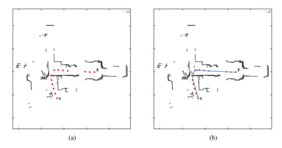
Figure 3.6: (a) Albot1's trace map consisting of 13 red points. (b) Albot1's simplified trace map consisting of only 4 points. Position '2' is regarded as an intermediate point for returning from '1' to 'S' and thus avoiding the obstruction.
