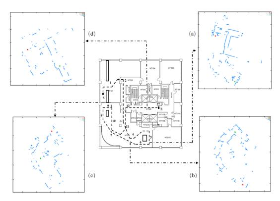
Figure 3.12: The environment and the path. The numbers indicate the travel direction. (a), (b), (c), (d) are four egocentric maps computed while exploring the environment.
