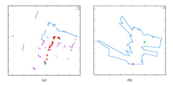
Figure 4.1: (a) Albot1's egocentric map before turning around. The purple lines indicate the part where the incoming view will cause an overlap (b) Albot1's enduring map which is a copy of the egocentric map shown in (b). Its boundary is computed using the algorithm: http://www.angusj.com/delphi/clipper.php.
