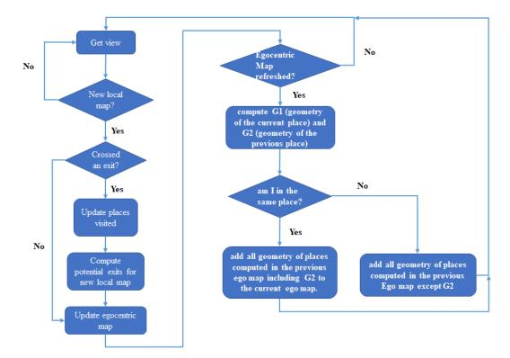
Figure 4.28: shows the flowchart for the new mapping process and algorithm is as shown below.
