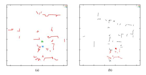
Figure 4.11: (a) The egocentric map computed prior to turning around at point 1. (b) The enduring map computed and re-aligned with Albot1's current view.
