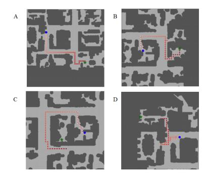
Figure 2.7: Four examples of computed maps using Gupta et al.'s system. In the map dark grey indicates occupied place and shadow grey indicates free space. In the maps, robot starts from the place of blue circle and targets to the position of green star. Red dotted lines indicate the path. (Reproduced from Figure 5, Gupta et al., 2017)
