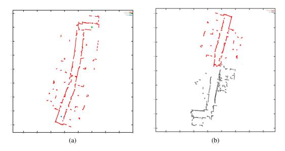
Figure 4.13: (a) The egocentric map computed prior to turning around at point E. However, for simplification, the display shows only the egocentric map computed from point 6 to point E. (b) The enduring map computed.
