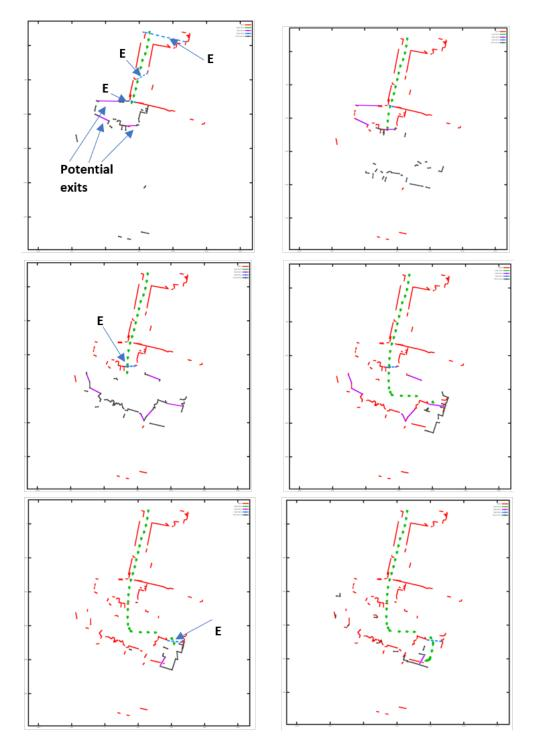
Figure 4.17: Computing places: (Left) Albot1 just crossed an exit (dashed blue line) and thereby identifying the current local map as a place and its potential exits (purple lines) are then computed. (Right) Albot1 moved inside a place, computing local maps as before. Each robot position (green dot) indicates a local map is being computed.
