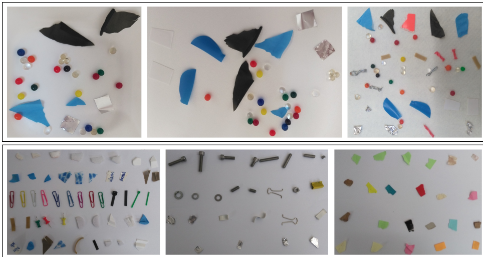
Figure 6.1: Top : Examples of used foreign materials in training and validation images. Bottom : Set of materials used in testing images.
