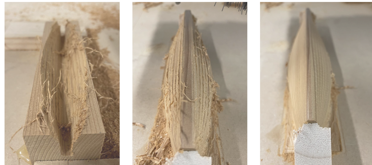
Figure 17,18,19,20. Davis, M. CNC. Western red cedar 2022 CNC as sketching through toolpathing: roughing in / finishing and exploration of grain qualities
