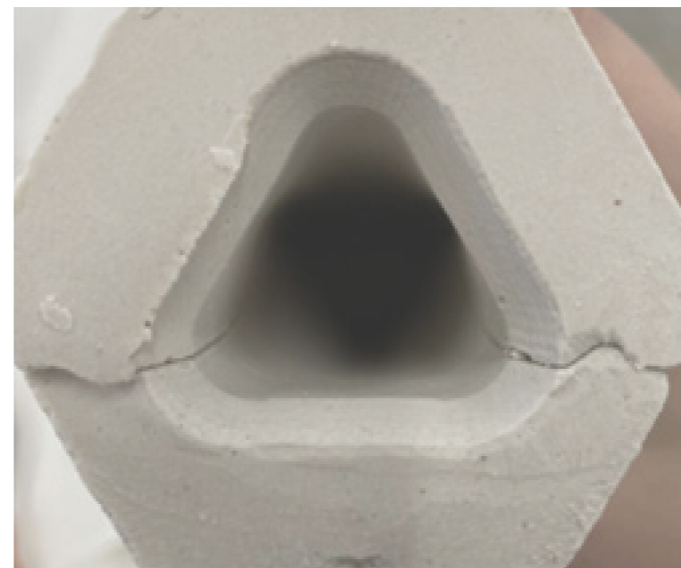
Figure 33. Davis, M. Digital. 2022 Slip mould detail showing artifact from digital part lines
