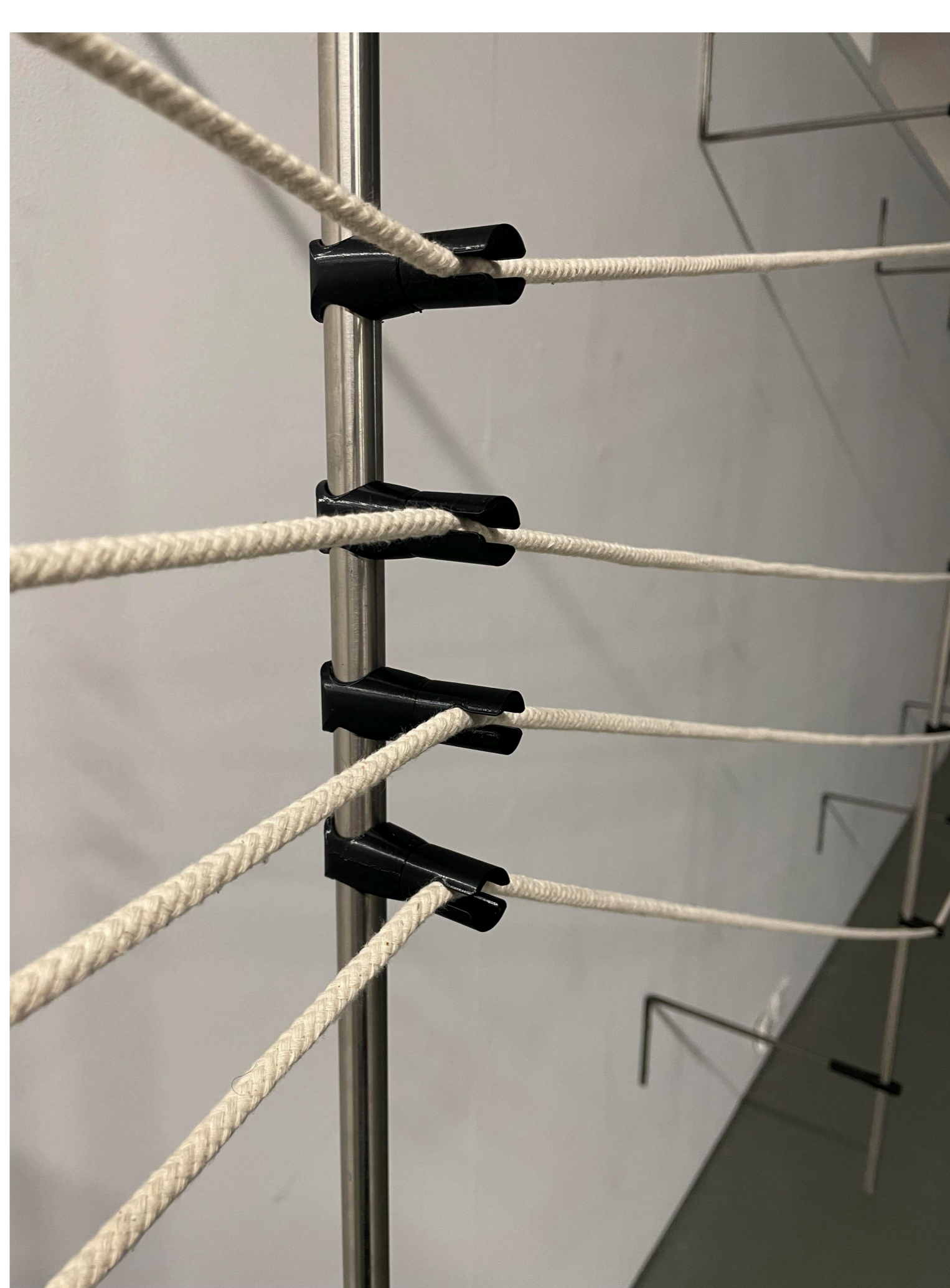
Figure 50. Davis, M. 'Interface 1'. Rope, 3d printed PLA, Steel rod. Test space WM level 2, 2022 Juncture detail of nodes and rope interacting
