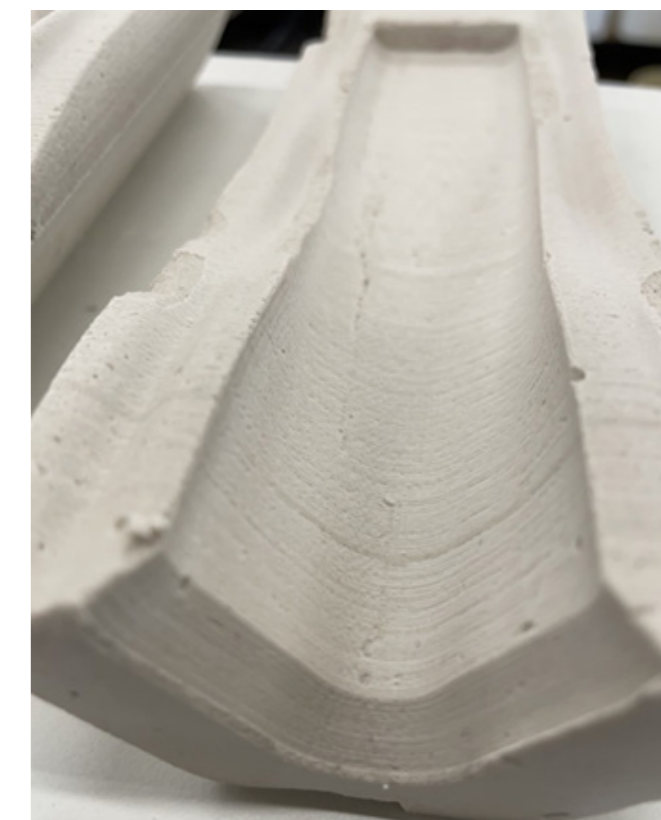
Figure 34,35. Davis, M. Digital. 2022 Tectonic strata of slip mould artifact of 3d printing
