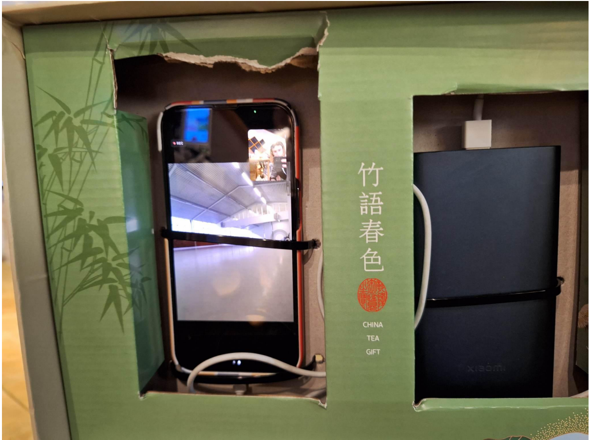
Figure 10. The 'DIY telepresence trolley'. (Image supplied by the authors).
