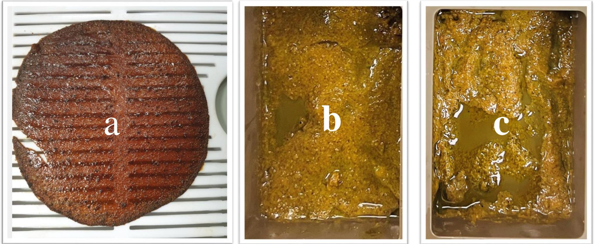
**Figure 33.** Avocado film created using 0.3 g dried avocado peel (a), 3.7 g dried avocado peel (b) and 7.4 g dried avocado peel (c).
