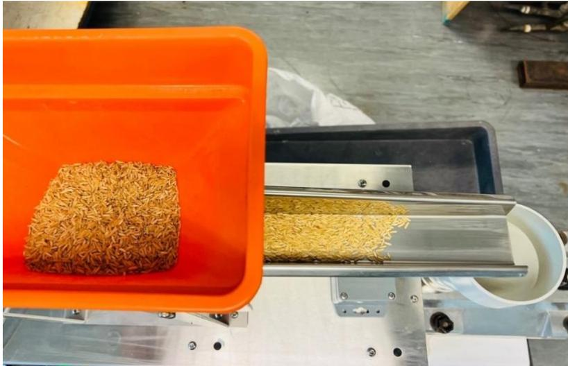
**Figure S-21.** Vibration feeder filled with brown rice, that will feed down the extrusion hopper and into the extrusion chamber. Feed flow rate was fixed at 5.3, 13.1 and 12.8 kg/h for avocado seeds, brown rice, and barley respectively.
