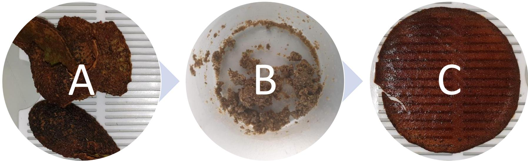
**Figure 32.** Conversion steps of avocado peel into film. Freeze dried avocado skin (A), Powdered freeze-dried avocado skin, mixed with 1.6 g distilled water (B), and film created using Ca-Zn- avocado skin mixture (C).
