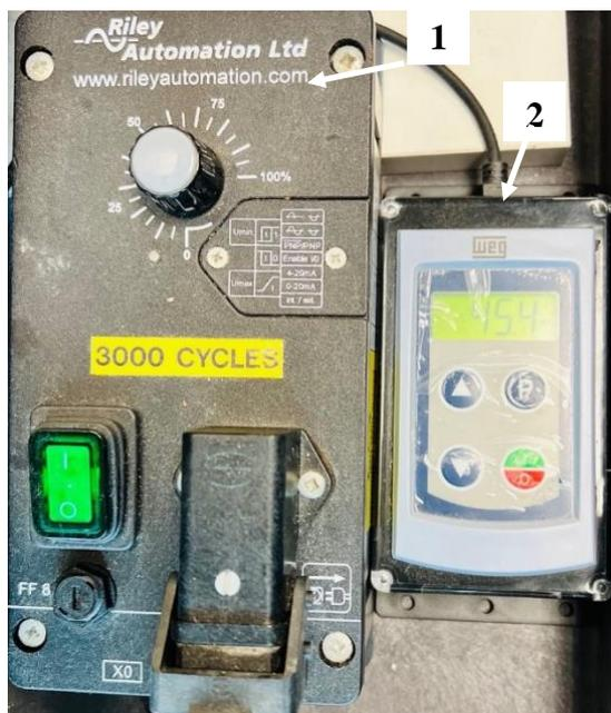
**Figure S-23.** Control box for vibration feeder (1) and control panel for screw shaft (2).
