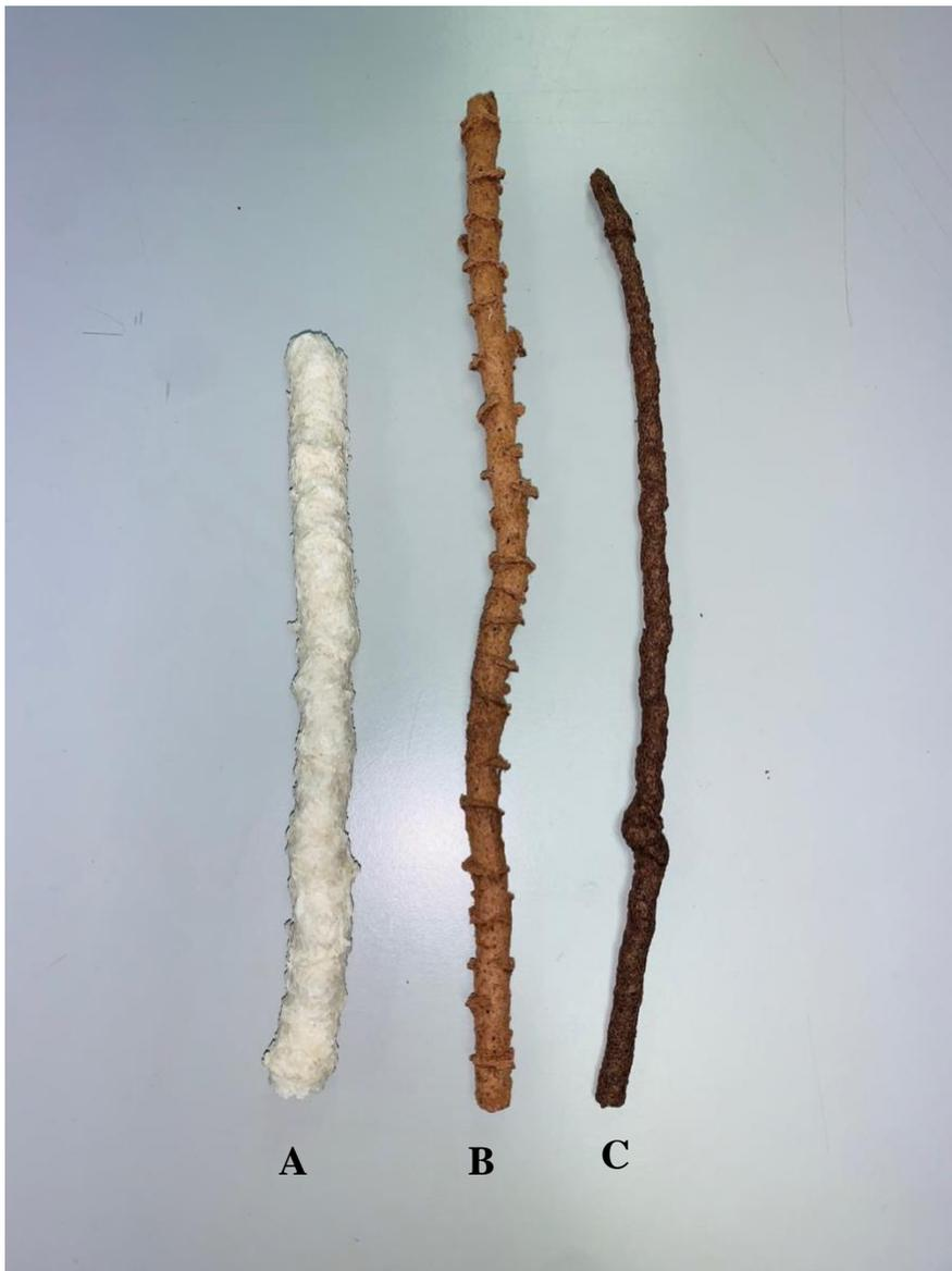
**Figure 16.** Brown rice (A), malt barley (B) and avocado seed (C) extrudates produced from the friction cooker Zapmill™ under the following conditions: Feed flow rate 12.8 kg/h (brown rice), 13.1 kg/h (barley) and 5.3 kg/h (avocado seed); Screw speed 50 Hz; 5 mm die opening.
