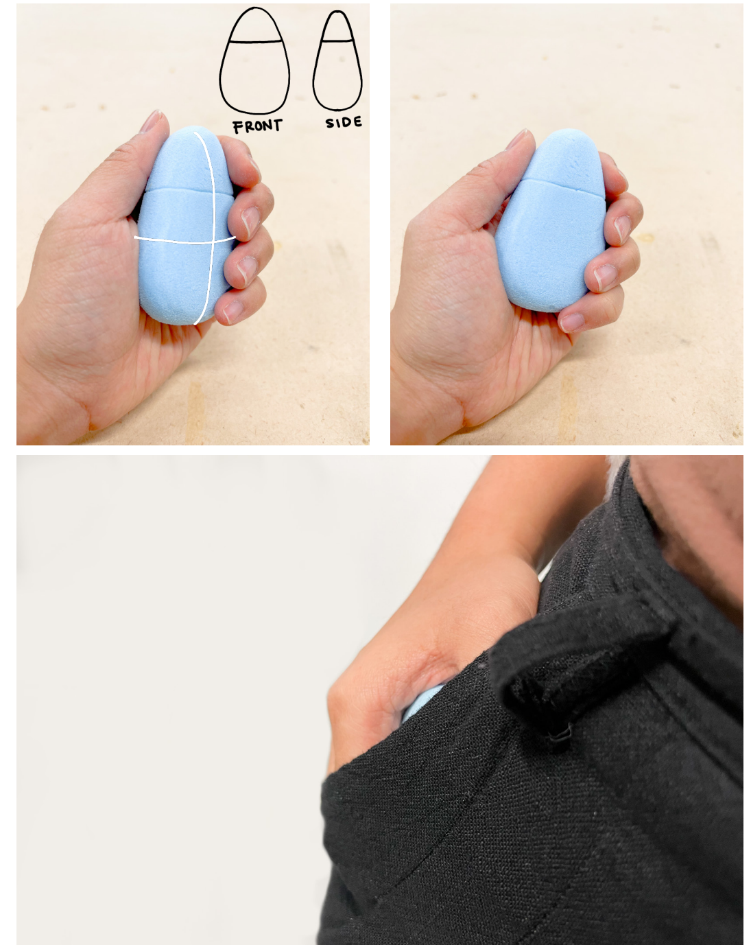
Figure 64 – Prototype three: the smaller size made this prototype easy to grip. In contrast to Prototype 2, the shape made it intuitive for the user to know where the top and bottom of the device would be. The slightly larger width at the bottom made it more secure in the palm of my hand.
