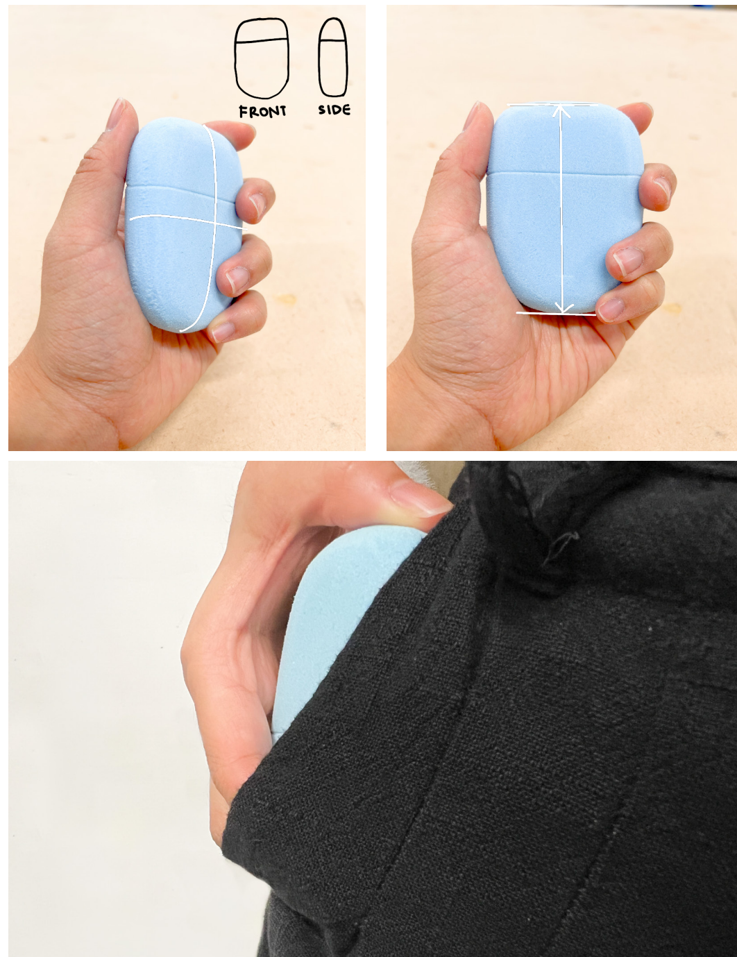
Figure 67 – Prototype six: I experimented with a slightly larger size and found it was more difficult to fit and carry around in a pocket. It was comfortable to grip, but from this I had to reconsider the size of the refined concept and find a balance.
