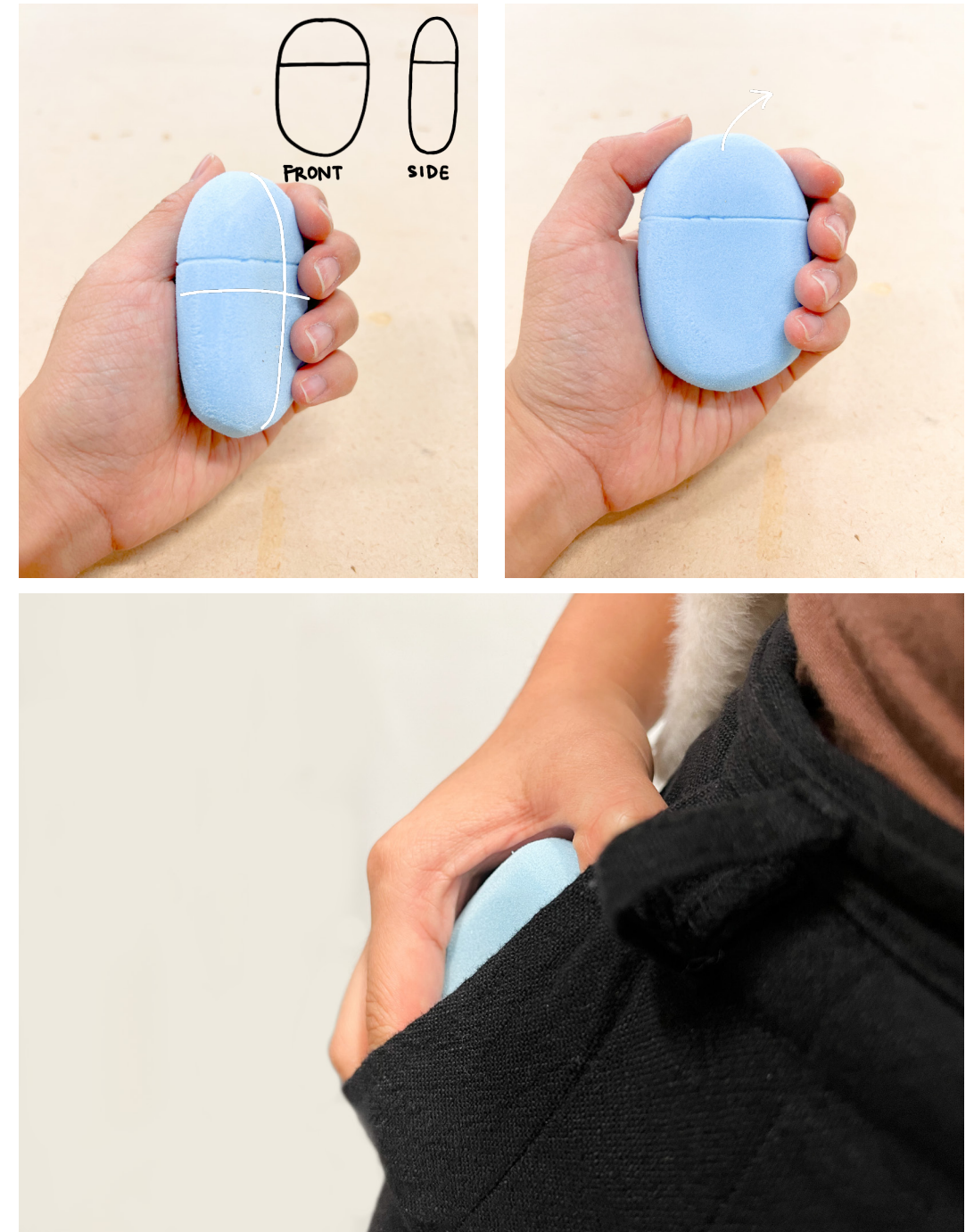
Figure 62 – Prototype one: this was the most “geometric” shape of the six prototypes, resembling most like a rectangular ellipsoid. It did feel stable in hand and easy to pocket, but due to its symmetric form, the user would not be able to recognise where to place their hand around the device instantly.
