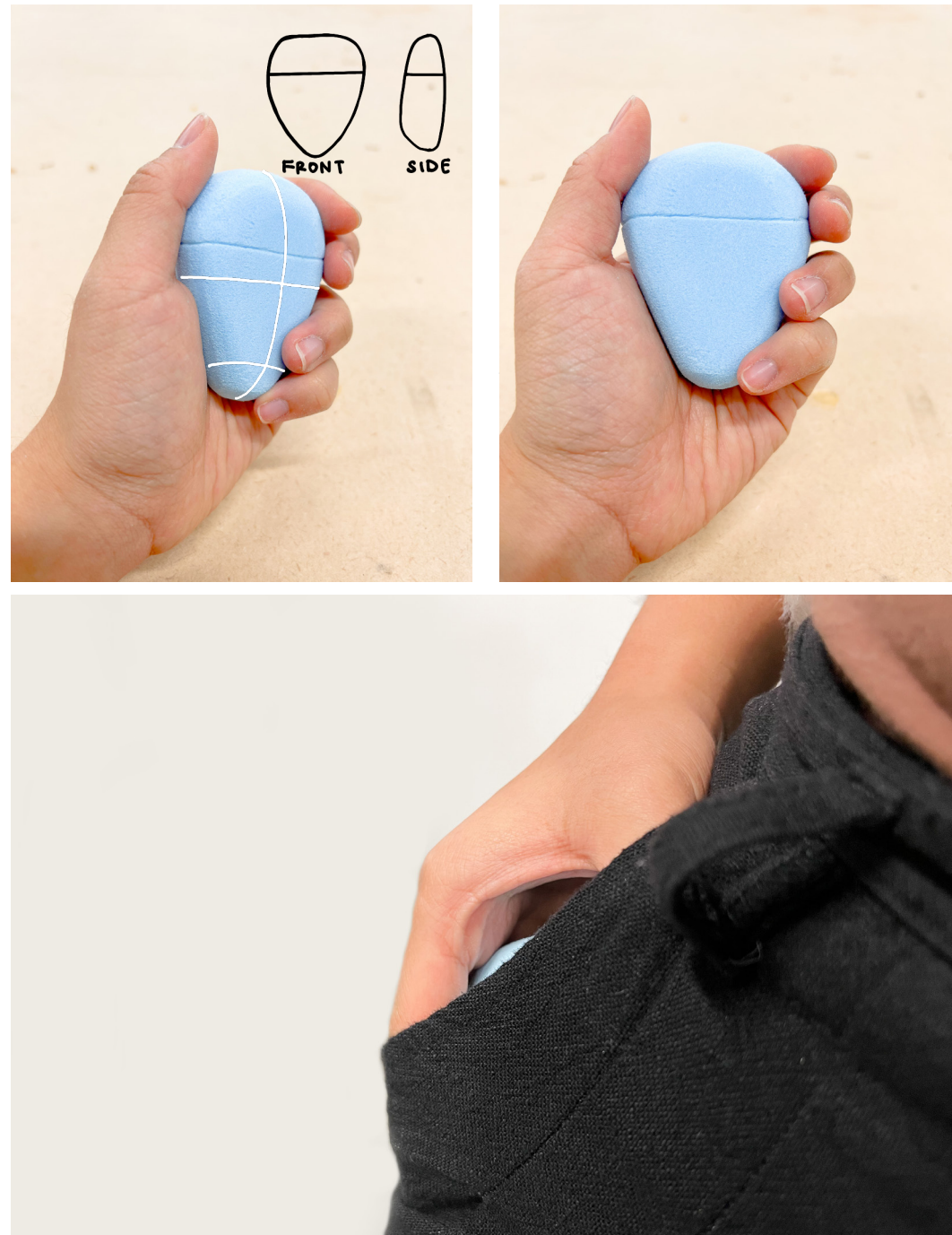
Figure 63 – Prototype two: I attempted to test a form with the pointed end as the bottom of the device. I realised it did not feel as comfortable as the other way around, although the slight outward curve for the back of the device made it feel more intuitive to know how it should be held. The pointed end at the bottom may confuse users, as it looked more natural for the point to be at the top of the device.
