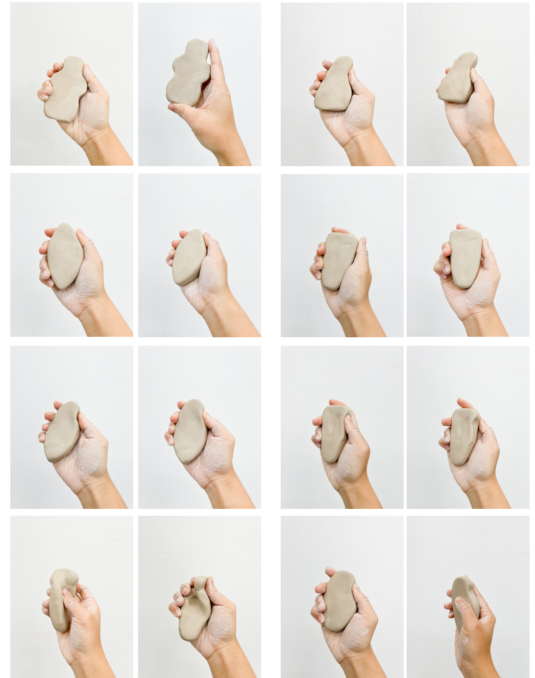
Figure 41 - Experiment with organic forms for the body of the inhaler through clay models.
