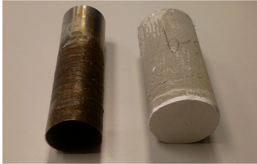
Figure 2.5.9 Cylindrical tubes used for cuff pressure calibration. The lightweight form concrete on the right hand side of the picture was used for large cuff calibration. The metal cylinder on the left hand side was used for medium and small cuffs calibration.
