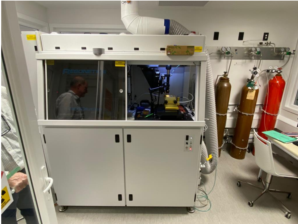
Figure 2. 6. Picture depicting the Applied Spectroscopy RESOLUTION M-50 laser ablation instrument.
