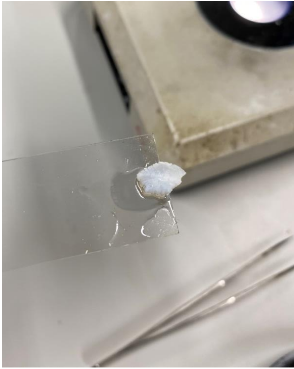
Figure 2. 2. Photograph of the otolith preparation sequence depicting an otolith glued hanging over the edge of a slide ready for the initial grind.
