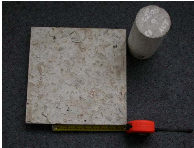
Figure 29: Slab of mussel shell-containing concrete used in the thermal properties determination.
