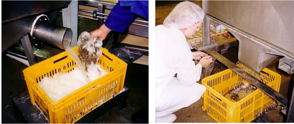
Figure 5: Byssus-waste catching bins at two different mussel-processing factories (Photo: Barnaby, 2002).
