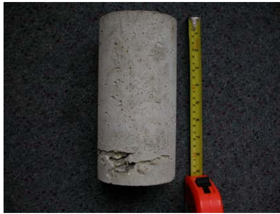
Figure 26: A test cylinder used in the compressive strength determination.
