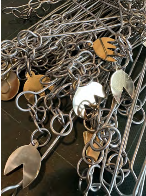
Figure 44. Jo Bradbeer, Surveyor's Chain Replica (October 2025). Steel and brass (66 feet - 20.1m - 100 links) and Chris Bradbeer using the chain to measure the length of Upland Road Track (22 March 2026)
