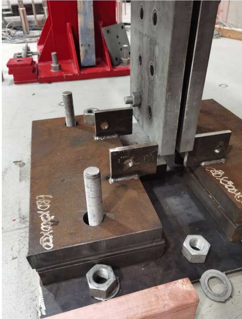
Figure 71: Placing the cover plates on the test sample (flange base plate)
