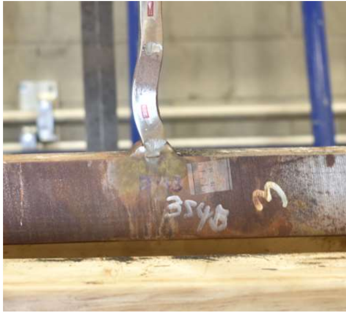
Figure 101: Failed (terminated) in Slipping of the test sampleFW10G0R0N3S4
