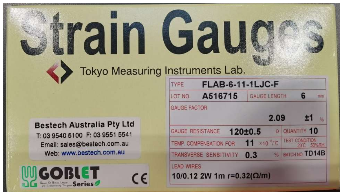
Figure 52: The details on the package of strain gauge from Bestech Australia Pty Ltd
