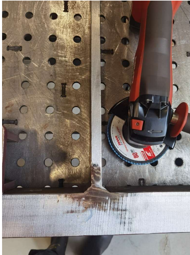
Figure 85: Finished steel surface after 80-grit grind
