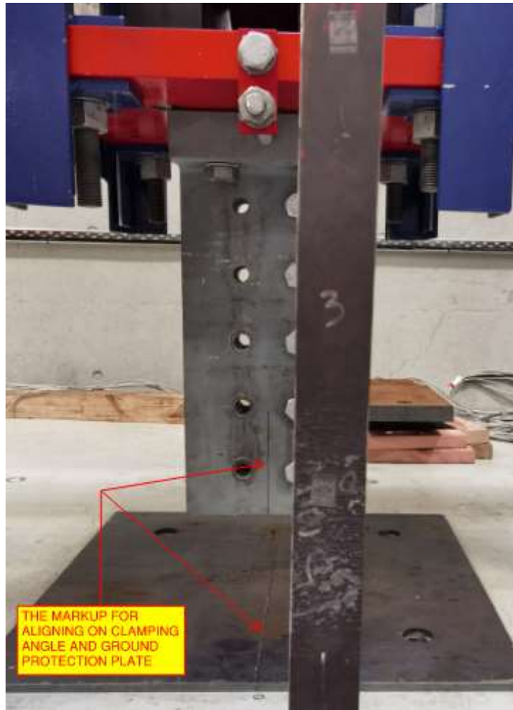
Figure 68: Marked up central lines on the clamping angle and ground protection plate for alignment purpose
