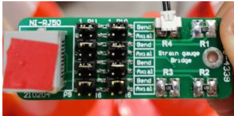
Figure 64: The circuit board for quarter bridge connection
