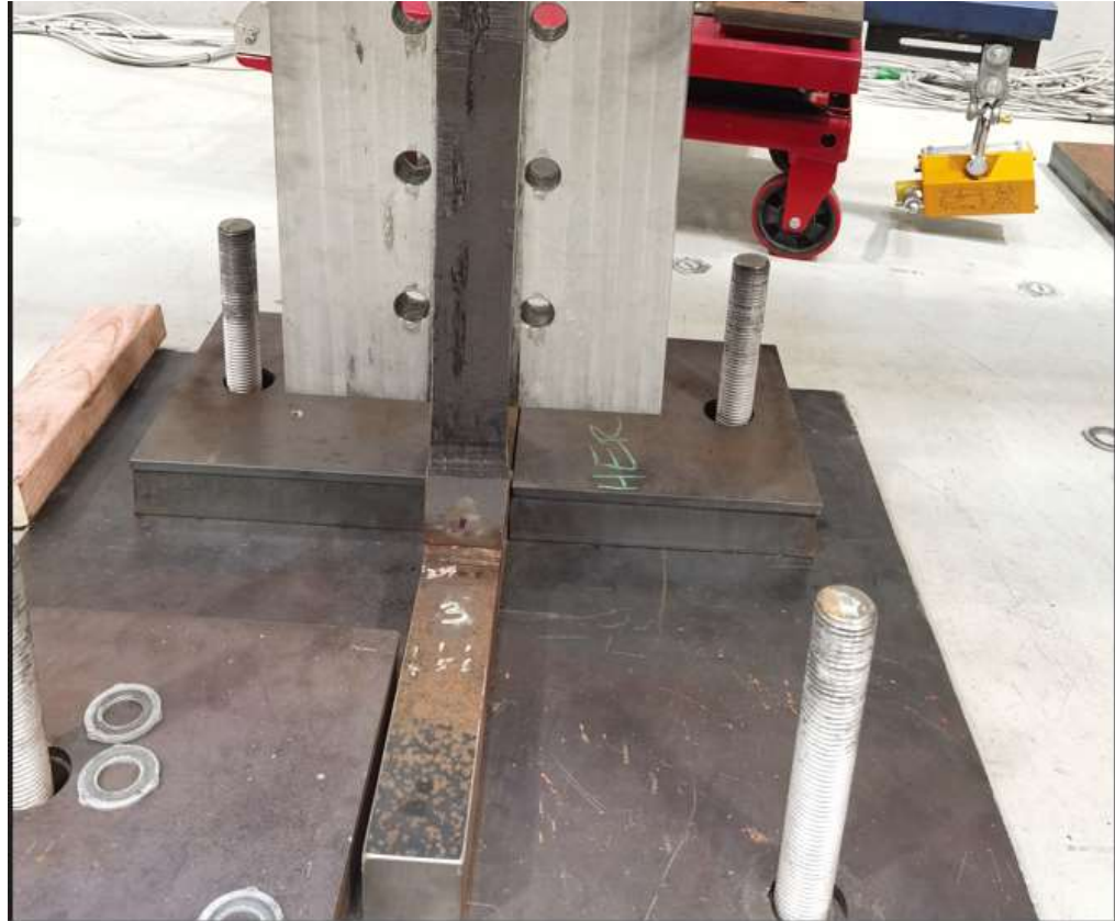
Figure 70: Placing the test sample in a position close to one of the clamping angles.
