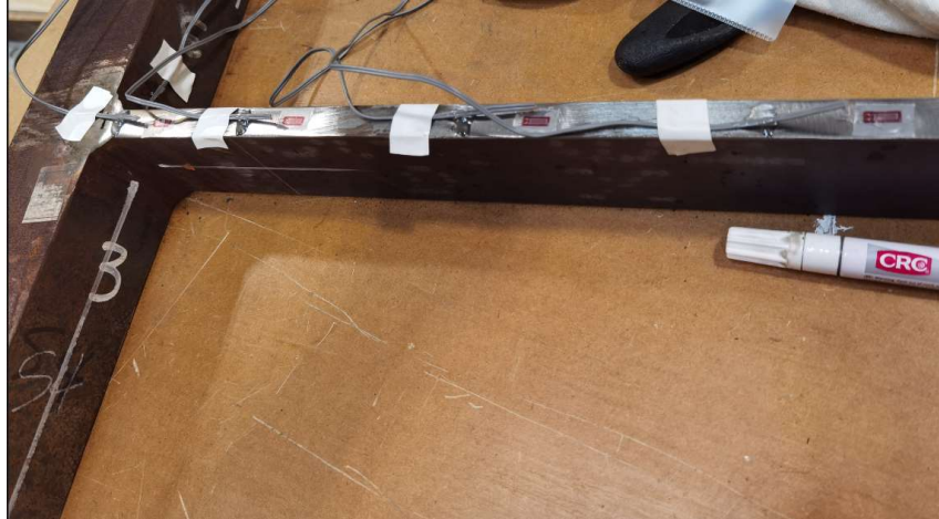
Figure 66: The sample with strain gauges installed
