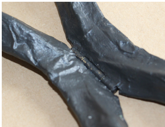
Figure 83: Artefact D.2 – Hinge joinery mechanism
