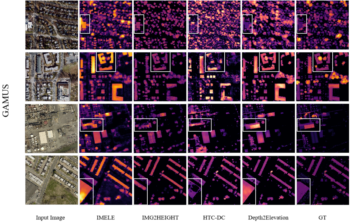
Fig. 5. Qualitative comparison on the GAMUS dataset. Compared with other methods, Depth2Elevation predicts the height and integrity of buildings more accurately and depicts the subtle height changes of roofs more carefully.
