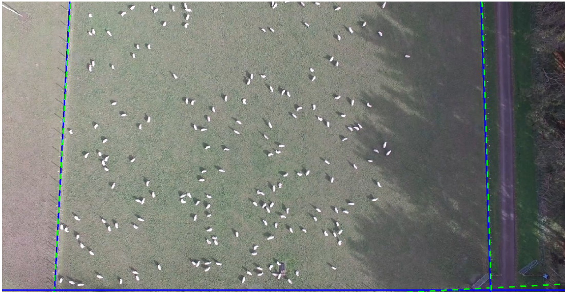
Figure 6.7: Estimated and actual fence lines shown in blue and green respectively for the 5 th frame of 80b.
