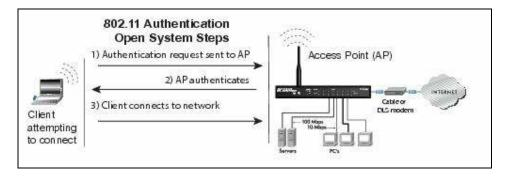
Figure 2.2 802.11 Open system authentication (Netgear Inc, 2005a)
