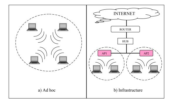
Figure 2.1 WLAN architecture a) Ad-hoc (IBSS) and b) Infrastructure (ESS)
