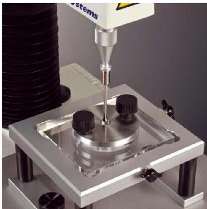
Figure 3.2. The film support rig with 5 mm spherical probe placed on TA.TX *Plus C* Texture Analyser (Adopted from (Smewing, 2015)).
