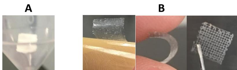
Figure 5.6. Effect of drying technique on 10% GelMA hydrogel meshes. Fragile freeze-dried meshes (A), and easy to handle vacuum-dried meshes (B).
