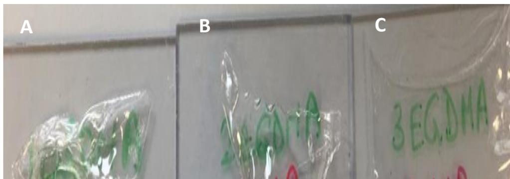
Figure 3.4. The effect of the crosslinker concentration on silicone hydrogel films containing 0.75 mole% PDMS, 10 mole% TRIS and 0.5% LAP. Films shown had EGDMA concentrations of either 1% (A), 2% (B) and 3% (C).
