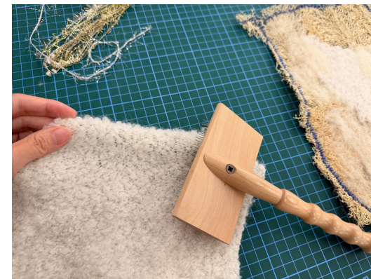
Figure 4.24 Brushing and loosening fibres from dismantled textile samples during the reconstruction process. Researcher's personal archive.
