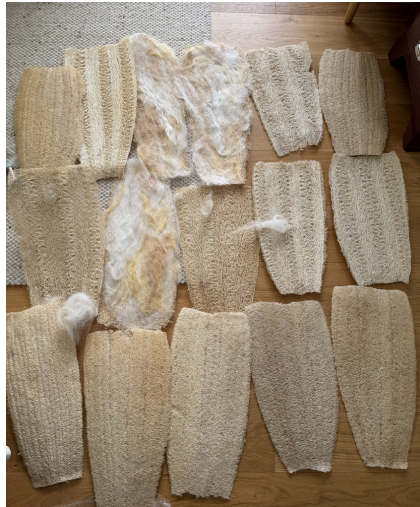
Figure 3.3 Early material testing comparing variations in loofah form, colour, and structure, alongside layering experiments with wool felt. These comparisons helped identify how differences in material density and combination could inform subsequent material decisions. Researcher's personal archive.
