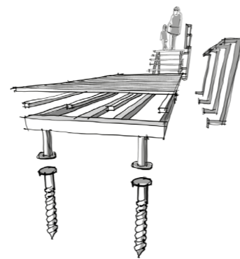
Fig. 16 Isthmus, The boardwalk is founded on steel screw piles , Digital Drawing, 2020, (Isthmus, Auckland), https://isthmus.co.nz/project/maungawhau-boardwalk/
