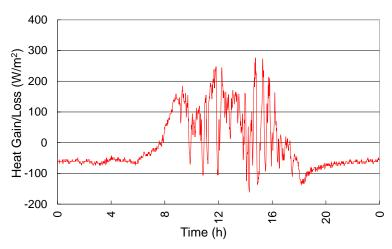
Figure 3: Heat transfer to and from the collector
