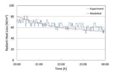
Figure 4: Cooling provided by radiant cooling panel
