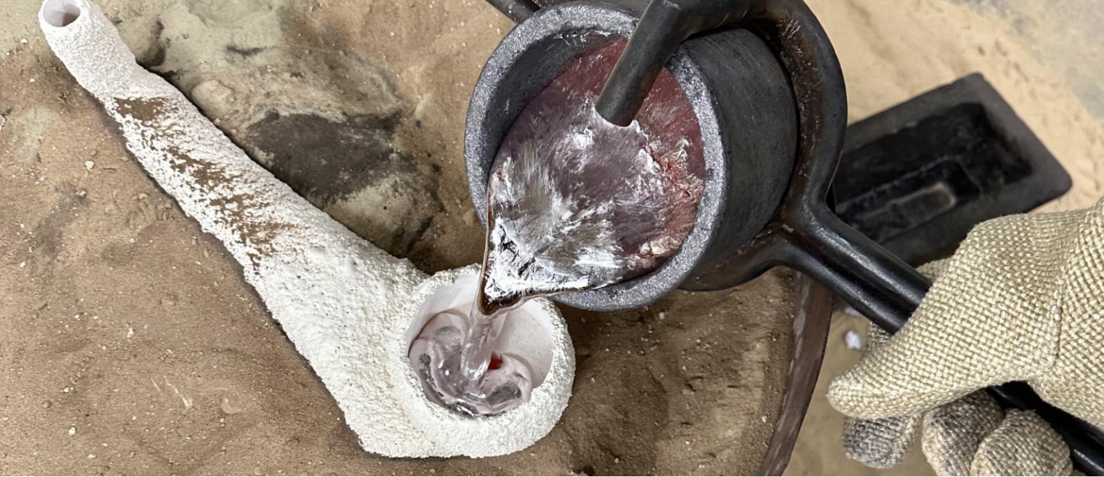
Figure 50: Above is a stage when aluminium is poured into the cast, once the 3D print has melted Figure 51: Below is a series of Axial Rod head in aluminium
