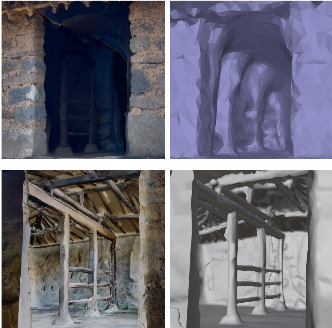
Figure 69. Comparison between videogrammetry (top) and MLS (bottom) results. Videogrammetry shows a realistic look of the textured mesh (left), but the solid view mode (right) makes insufficient mesh generation apparent. In contrast, the MLS result shows a more detailed mesh and overall higher accuracy of the structures.
