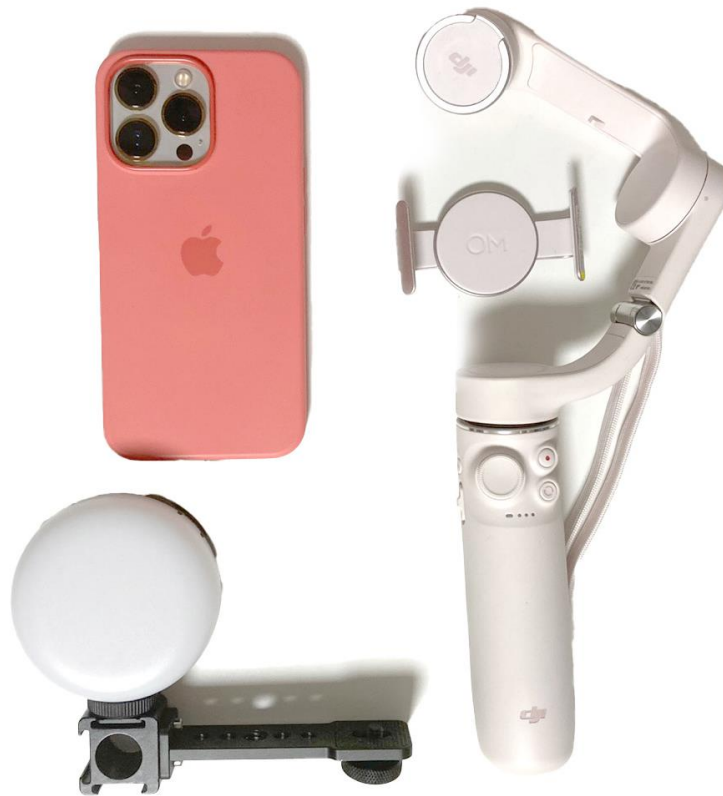
Figure 55. Capture equipment for videogrammetry and MLS (top left: iPhone 13 Pro, right: Handheld gimbal, bottom left: external LED light)
