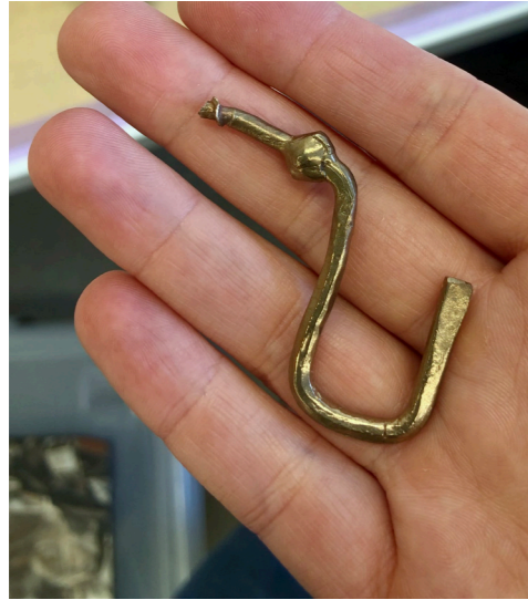
Image 247. Emelia French, custom bronze hook, 2022. This one snapped in the wall because the bronze was too malleable.
