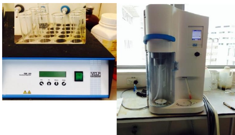
Figure 6 Velp DK 20 heating block for digestion and VelpUDK 139 distillation unit used for protein analysis
