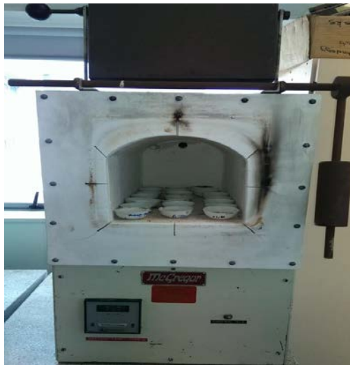
Figure 7 Muffle furnace set at 550°C for ashing of bread samples
