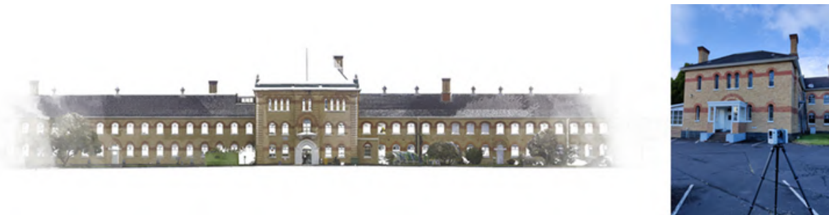
Figure 8. Point cloud image of the main façade of Building One, Generated by the Digital Heritage Research Centre at Unitec (Milic, 2024).
