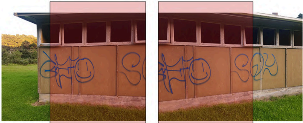
Figure 9. Example of two photos of the target object, taken with a minimum overlap of 40%, by Author
