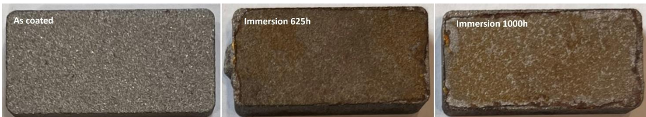
Fig. 3 Photographs of the uncoated and sandblasted sample as blasted and after 3.5 wt% NaCl for 625 hours and 1000 hours
