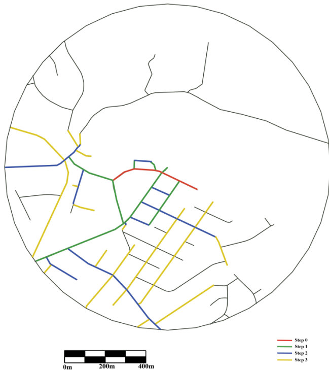
Figure 4.89: Three-step connectivity analysis for Baxter Street in the Warkworth suburb in Auckland (by author).
