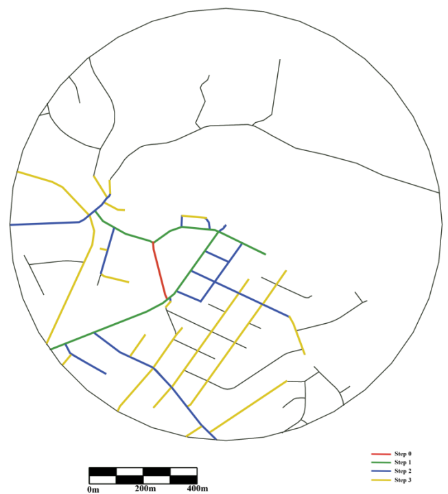
Figure 4.90: Three-step connectivity analysis for Twin Coast Discovery HWY in the Parnell suburb in Auckland (by author).
