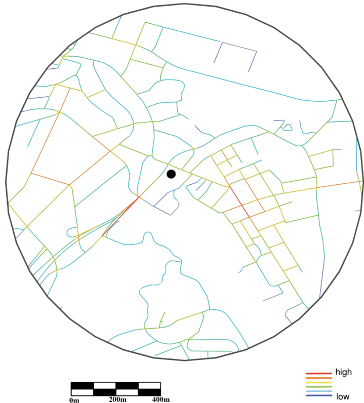
Figure 4.38: Local integration analysis for the Parnell suburb in Auckland with the main street of Stanley Street as the root node (by author).
