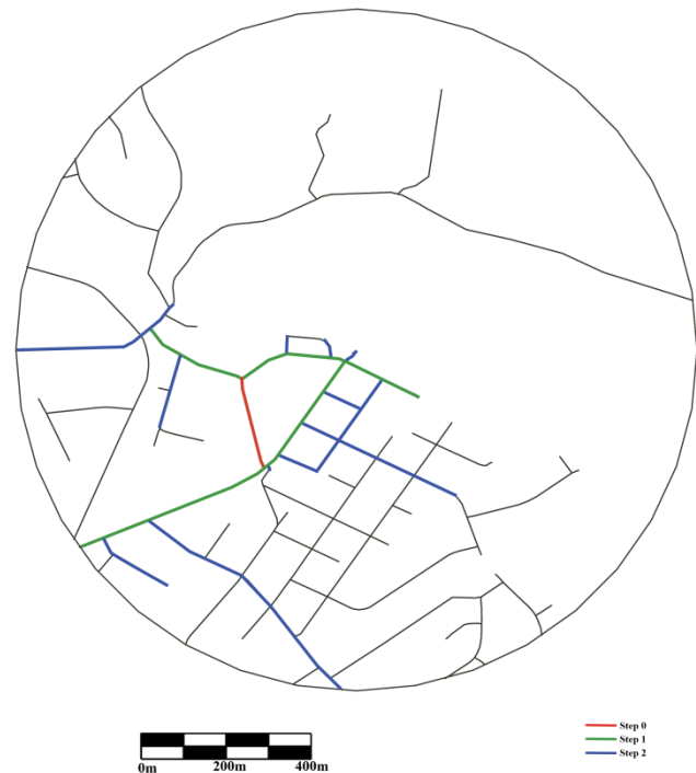
Figure 4.87: Two-step connectivity analysis for Twin Coast Discovery HWY in the Warkworth suburb in Auckland (by author).
