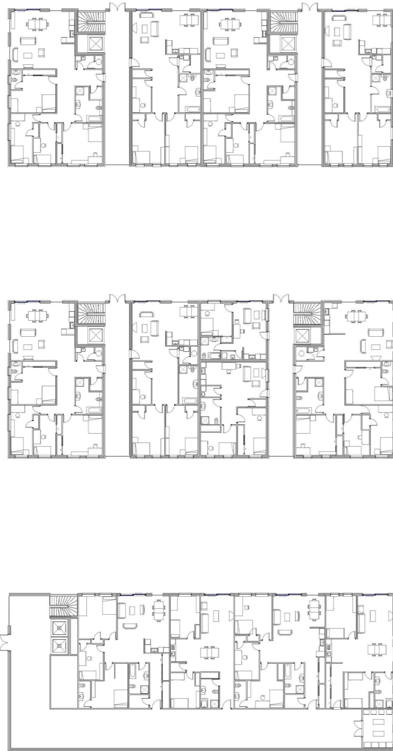
Figure 40. Early explorations of floor plans, considering sensory corridor (bottom), and separated apartment layout (top and middle).
